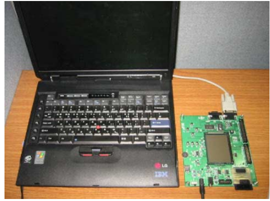
Fig. 6. Prototype of SmartMedia Card with the flash compression layer.
