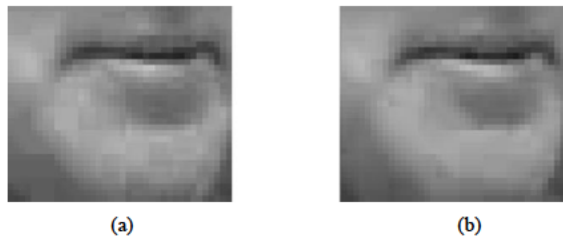
Fig. 1. Detail of luminance input to the deblocking filter in the case of (a) loop-filtering and (b) post-filtering based system.
