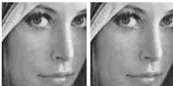
(e) DCT(QS), 0.3 bpp ( q = 17.95 ), PSNR = 32.22 dB
