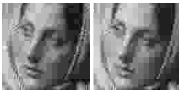
(e) DCT(QS), 0.15 bpp ( q = 5.07 ), PSNR = 23.58 dB
