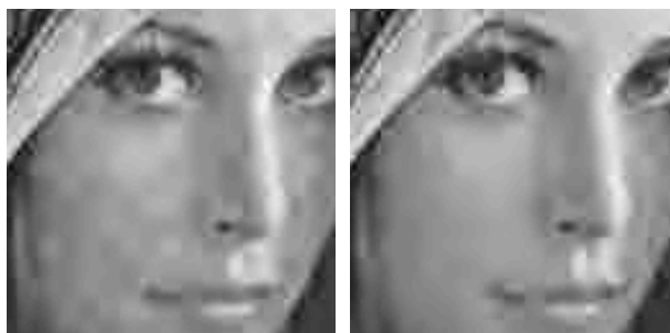
(c) PPHLCT(QS), 0.15 bpp ( q = 7.35 ), PSNR = 28.89 dB
