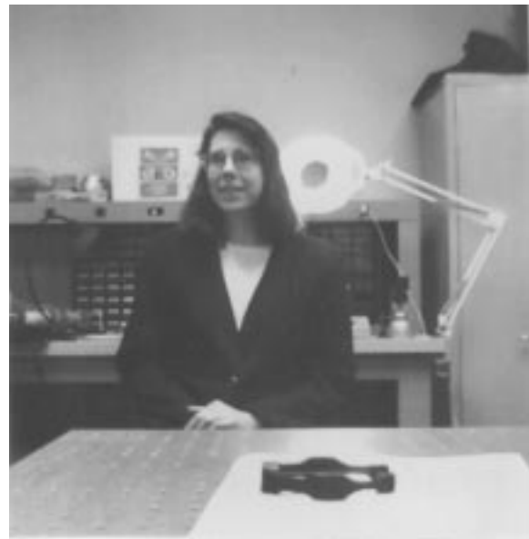
Fig. 10. Unprocessed image taken from a Photobit 256 \times 256 element sensor with on-chip ADC operating at 30 frame/s. Note no blooming from light and lack of other artifacts.
