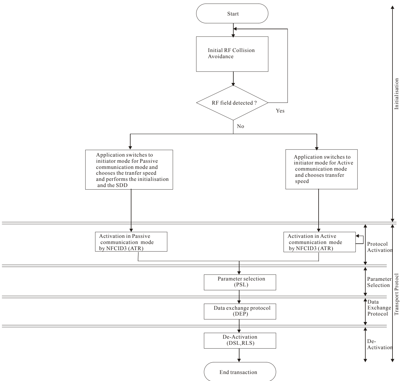
Figure 5 – General initialisation and single device detection flow
