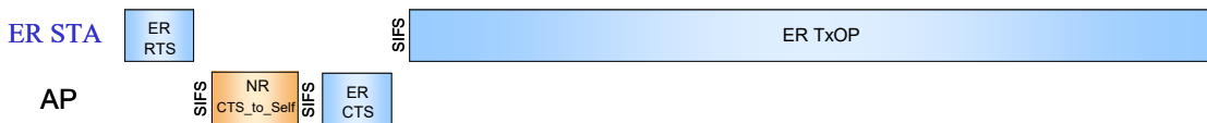
41 42 Figure xxyz3: Protection of an EDCA ER TxOP initiated by a non-AP 802.11n STA
