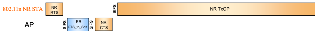
Figure xxyz4: Protection of an EDCA NR TxOP initiated by a non-AP 802.11n STA
