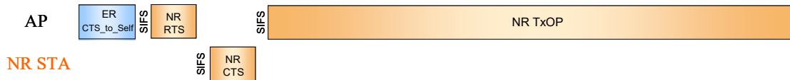
19 20 21 Figure xxyz1: Protection of an EDCA NR TxOP initiated by the AP (NR RTS and NR CTS are optional)
