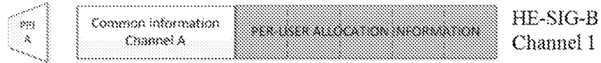
Figure 26 HE-SIG-B channel for 20MHz containing a common information followed by per-user allocation information
