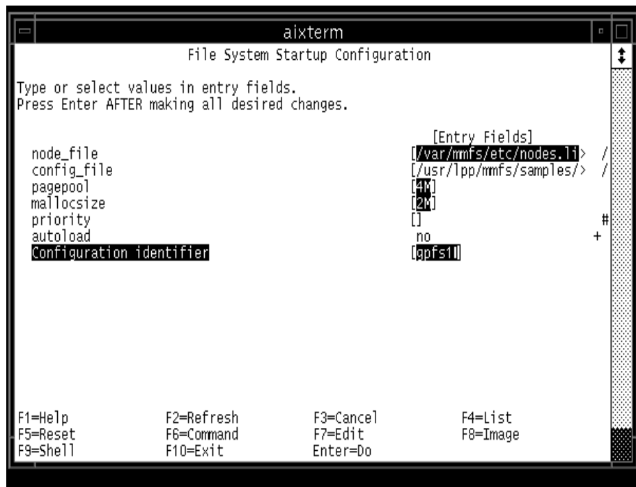
Figure 177. SMIT Panel for Configuring GPFS
