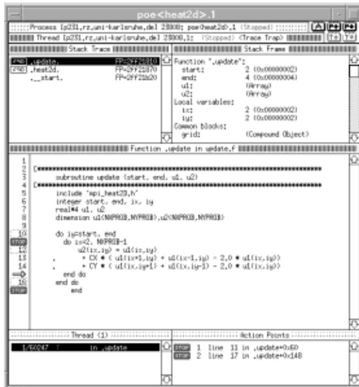
Figure 193. TotalView Process Window: Application Program
