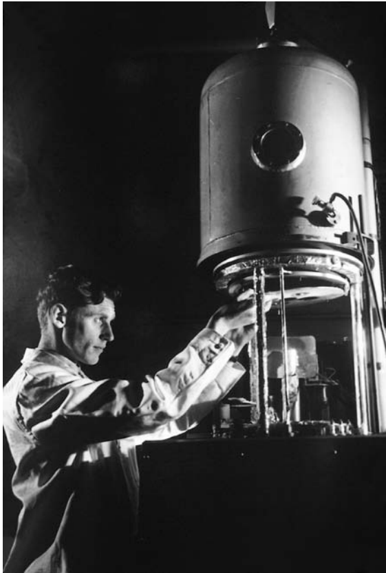
Preparing a plant for the manufacture of narrowband filters. (Courtesy of Walter Nurnberg FIEP FRPS, the editors of Engineering , and Sir Howard Grubb, Parsons & Co Ltd.)
