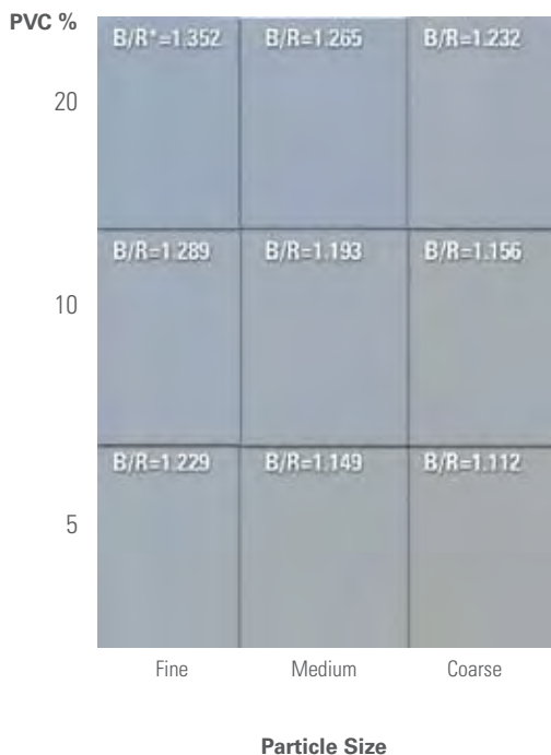
Figure 12. Titanium Dioxide Effect of Particle Size and PVC on Tinted Paint Undertone.
