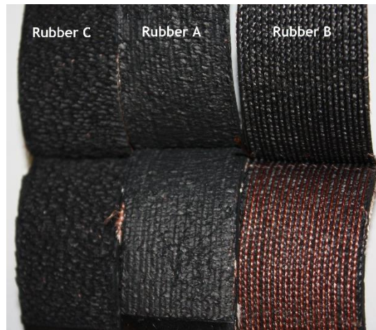
Figure 17 - Peel adhesion samples from the reference trials for nylon cord with dip I
