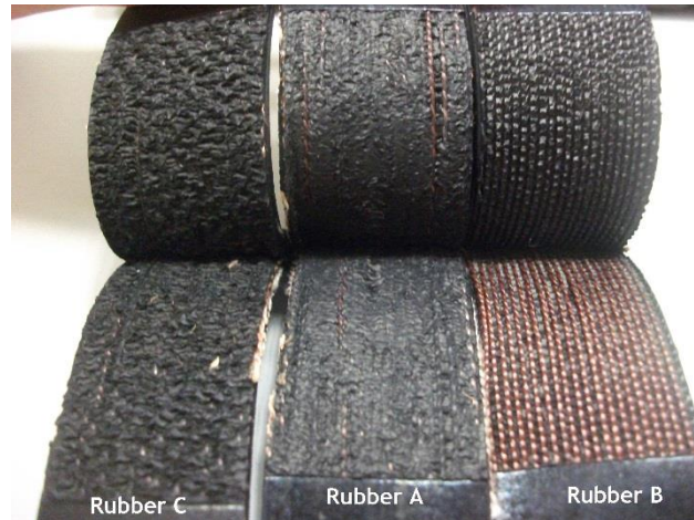
Figure 21 - Peel adhesion samples from the reference trials for hybrid cord with dip I
