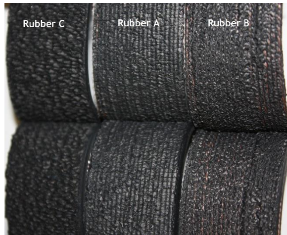
Figure 20 - Peel adhesion samples from the reference trials for nylon cord with dip II
