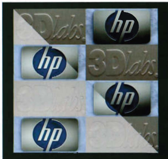
Color Plate 10 Image showing the difference between a conventional texture map (lower left) and a polynomial texture map (PTM) (upper right). The conventional texture looks flat and unrealistic as the light source is moved, while the PTM faithfully reproduces changing specular highlights and self-shadowing. (© Copyright 2003 Hewlett-Packard Development Company, L.P., Reproduced with Permission)
