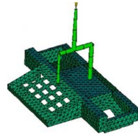
Fig. 21. The runner system
