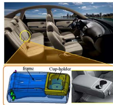
Fig. 36. Rear center armrest with a cup-holder, [42]
