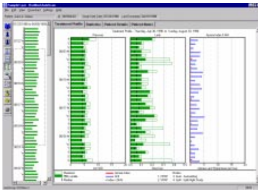
Treatment Profile – shows AH1, mask leak, and pressure requirements for 200 nights for optimizing long-term treatment efficacy
