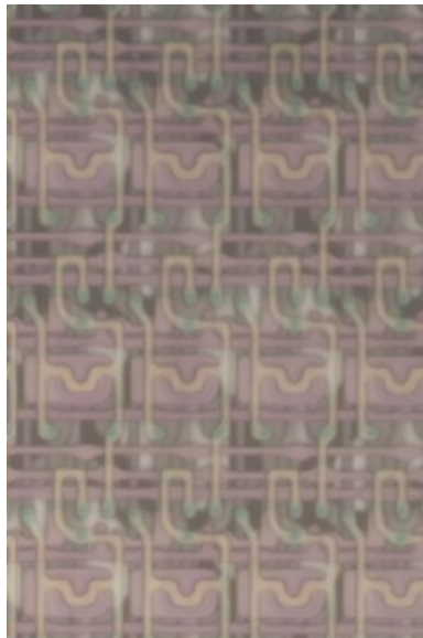
Optical image of OLED pixel structure, viewed from polysilicon side with poly-imide substrate removed, of BOE panel in iPhone 14.
