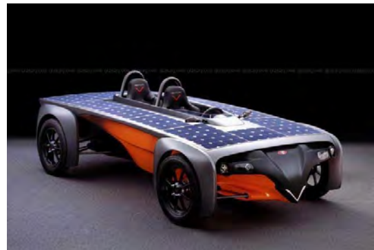
Pic. 2. Venturi Automobiles' Astrolab, the first commercially available PV integrated hybrid
