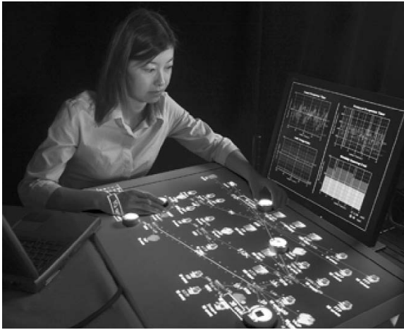
PHOTO 24.8. IP network design workbench running on Sensetable platform.
