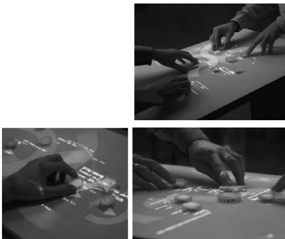
PHOTO 24.7. AudioPad running on Sensetable platform.
