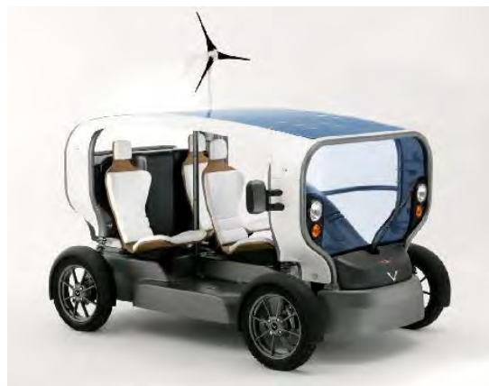
Pic. 3. Venturi Automobiles' Eclectic, the first energy autonomous electric urban commuter vehicle
