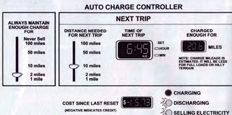
Figure 1: Suggested design of vehicle dashboard control, allowing driver to limit loss of range of vehicle and monitor power transactions.
