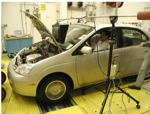
Figure 7. Prius emissions testing at constant output
