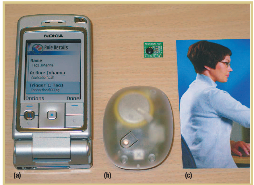
Figure 3. Pointing input. (a) After creating the rule, the device owner uses (b) a tag reader/writer to touch the RFID tag (the green chip) and call (c) the pictured person. The tag reader uses Bluetooth to connect to the phone.
