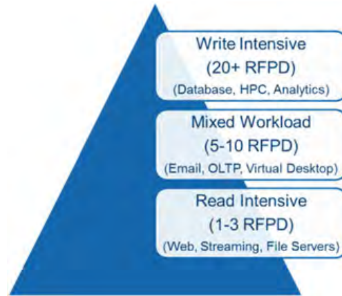
Fig. 1.4 Enterprise SSD usually classified in terms of an endurance metric and application space they target (RFPD—Random Fills Per Day for 3 or 5 years for cloud and enterprise usages is typically warranted). The traditional classification for enterprise SSD’s have yielded three distinct SSD drive specifications: “Read Intensive” at 1–3 RFPD, “Mixed Workload” at 5–10 RFPD, and “Write Intensive” at 20+ RFPD
