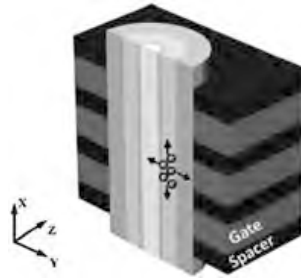
Fig. 2.18 3D CT-NAND structure and charge loss along X and Y axes [29]
