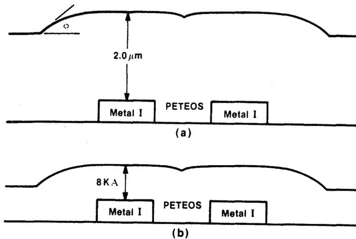
**Fig. 4-17** (a) Thick PETEOS deposition ( $2.0\ \mu\text{m}$ ) over  $0.5\text{-}\mu\text{m}$  Metal 1 creates a "smoothed" topography for Metal 2 at the edge of an isolated Metal 1 feature while planarizing closely spaced Metal 1 features. (b) An anisotropic etchback of the interlevel dielectric preserves the "smoothed" surface.<sup>37</sup> (© 1987 IEEE).
