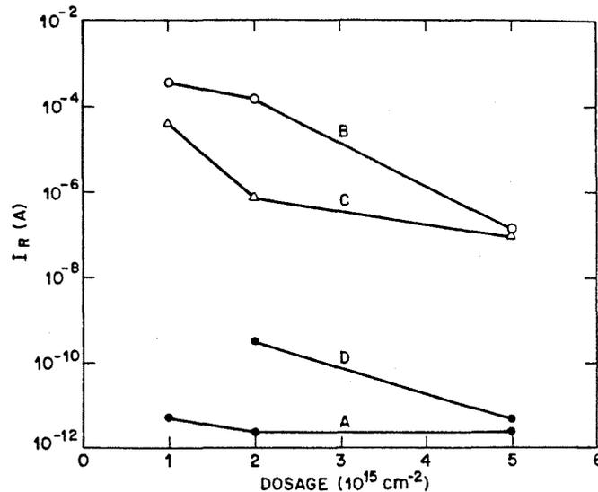
Fig. 3-44 Silicide junction leakage: (a) good  $n^+/p$  diode with no silicide, junction depth of  $0.15 \mu\text{m}$ ; (b) after forming  $0.07 \mu\text{m}$  of  $\text{CoSi}_2$ , Si consumed  $0.07 \mu\text{m}$ ; (c) after  $\text{CoSi}_2$  formation at  $700^\circ\text{C}$ , Si consumed  $0.11 \mu\text{m}$ ; (d) after a second  $900^\circ\text{C}/30 \text{ min}$  drive.<sup>96</sup> (© 1986 IEEE).
