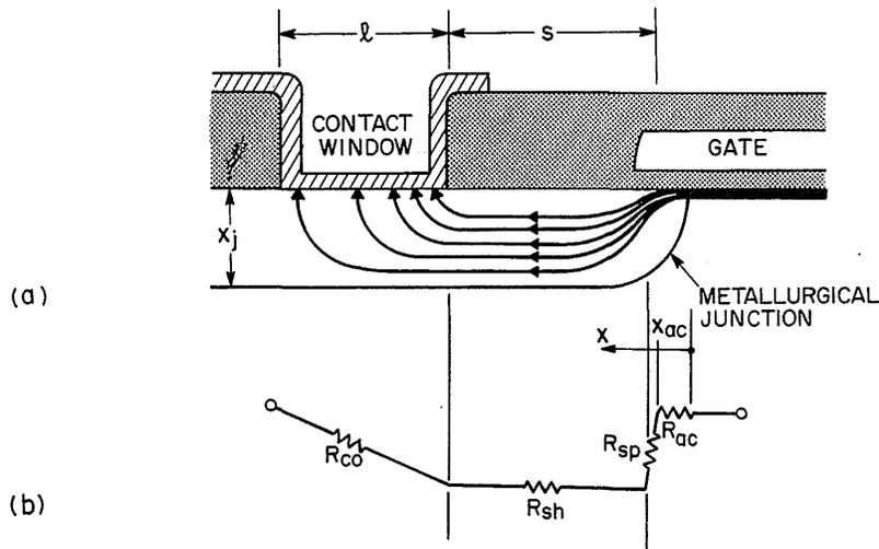
Fig. 3-1 Schematic drawing showing (a) current paths within the source and drain regions, of a planar MOSFET and (b) their corresponding representative series resistance components.<sup>84</sup> (© 1986 IEEE).
