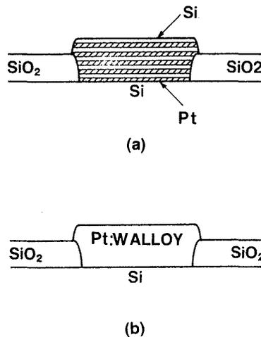
Fig. 3-25 Two approaches investigated to minimize the effect of excess Si consumption during PtSi formation: (a) the deposition of Si and Pt together, and (b) the deposition of an alloy of Pt and W.<sup>44</sup> Copyright 1981. Reprinted with permission of the AIOP.
