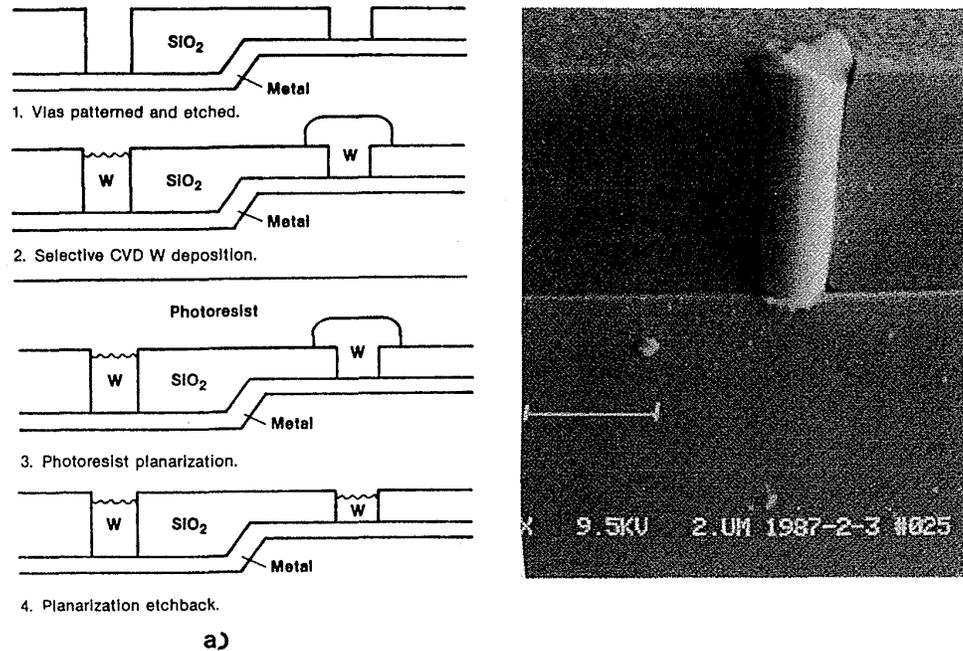
**Fig. 4-43** Method of forming metal plugs using selective W deposition, resist planarization, and etchback. The shallow openings are overfilled and must be etched back to obtain a planar surface. (b) An SEM photo of a via plug  $1.4 \mu\text{m}$  in diameter and  $2.2 \mu\text{m}$  deep formed by selective-W deposition.<sup>137</sup> (© 1986 IEEE).
