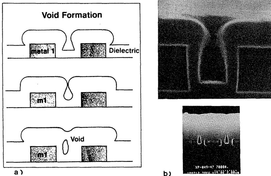
Fig. 4-8 (a) Diagram of void formation due to cusping of the dielectric. (b) SEM of voids left between 1.5- $\mu\text{m}$ -spaced Metal 1 lines in a 3.0- $\mu\text{m}$ -thick DM1 PECVD oxide.
