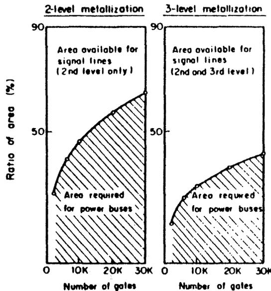
Fig. 4-6 Ratio of area required for power buses to the total chip area for ICs using two- and three-level-metal interconnect technologies.<sup>7</sup> (© 1983 IEEE).
