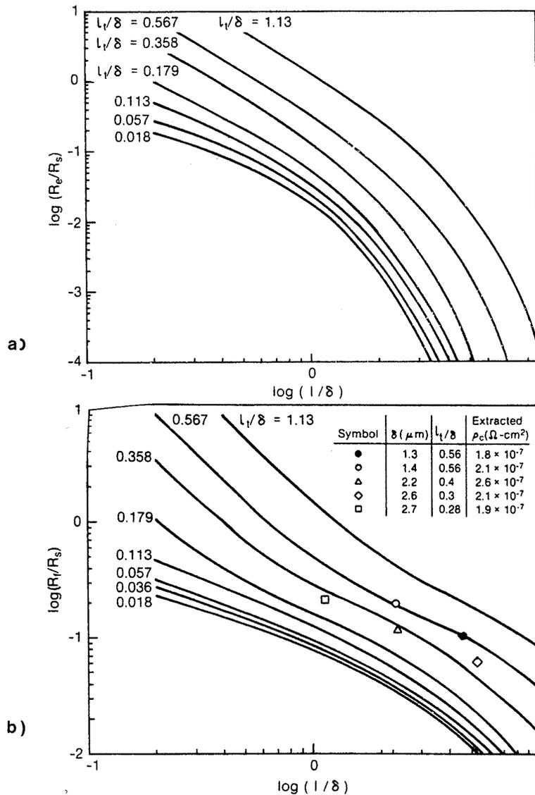
Fig. 3-11 Generalized universal curves for (a) the CER. (b) the TLTR. (Curves show  $l_t/\delta$  approximately in octave steps).<sup>7</sup> (© 1987 IEEE).
