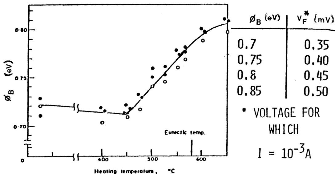
Fig. 3-33 (a) Barrier heights of Al-Si Schottky barrier diodes as a function of the heating temperature. (b)  $V_F$  (voltage at which the forward bias current in a Schottky diode = 1 mA) as a function of  $\phi_B$ .
