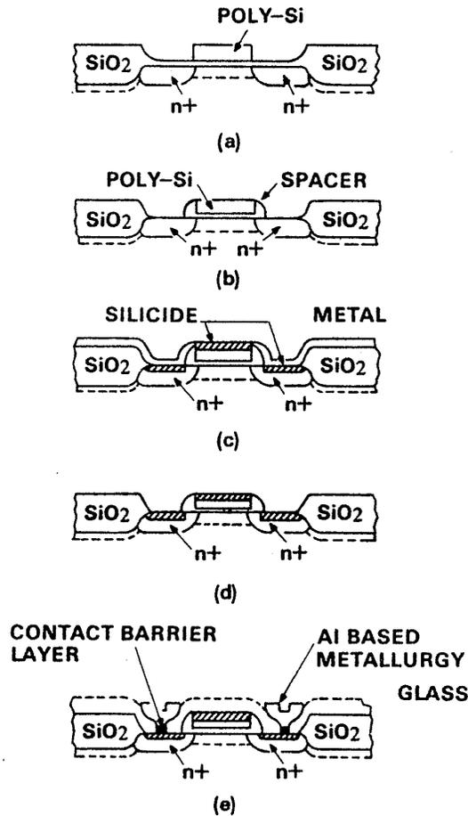
Fig. 3-39 Salicide processing steps and final structure.<sup>163</sup> (© 1984 IEEE).
