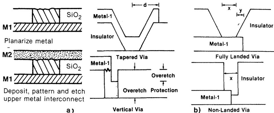
**Fig. 4-39** Metal 1 and Metal 2 pad areas can be smaller when vertical vias and fully filled vias are used because: (a) such filled openings provide protection during any overetch that may occur during the etching of Metal 1 or Metal 2; (b) any grooves that may be created during the overetching that occurs when the via openings are etched are easily filled by the via-filling process.<sup>128</sup> (© 1987 IEEE).
