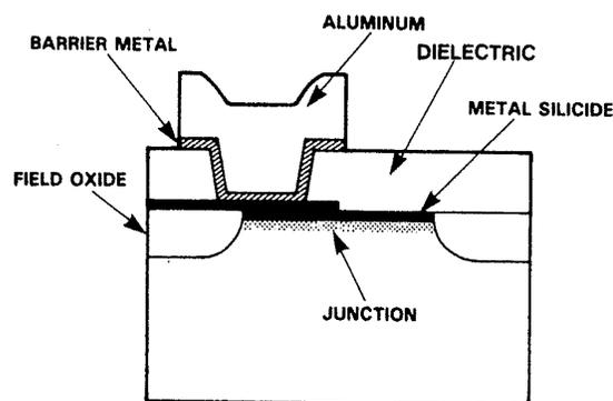
Fig. 3-53 HPSAC contact overlapping source-drain region and field oxide.<sup>122</sup> (© 1984 IEEE).
