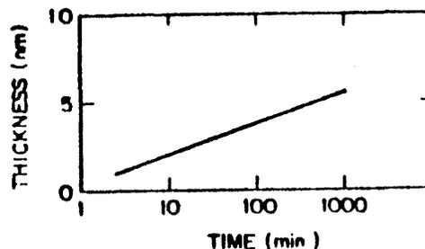
Fig. 3-15 Native oxide growth rate on Si exposed to room air.<sup>28</sup> Copyright 1984. Reprinted with permission of the AIOP.
