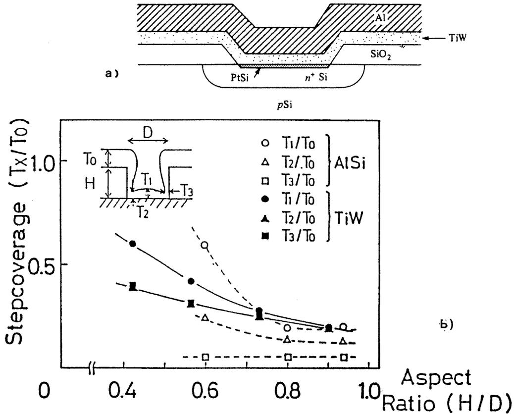
Fig. 3-27 (a) IC contact structure using Ti:W as a diffusion barrier to prevent reaction between PtSi and Al. (b) Comparison of the step coverage of Ti:W (0.6  $\mu\text{m}$  thick) and Al:Si (0.9  $\mu\text{m}$  thick) deposited into a 1.2- $\mu\text{m}$ -wide vertically sided, 0.9- $\mu\text{m}$ -deep contact hole.<sup>143</sup>
