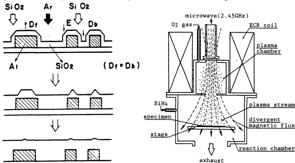
Fig. 4-34 (a) Principle of bias-ECR plasma CVD; (b) ECR plasma CVD apparatus.
