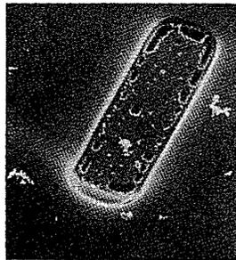
Fig. 3-22 SEM micrograph of Si pitting that exists after sintering of an Al-covered contact. (Al has been stripped after the sinter step.)<sup>165</sup>
