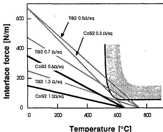
Fig. 3-40 Force at the silicide edge (silicide stress  $\times$  silicide thickness) versus temperature acting during cooling after silicide formation for the various samples. (Dotted lines correspond with samples in which defects are observed.)<sup>100</sup> This paper was originally presented at the Spring 1988 Meeting of The Electrochemical Society, Inc., in Atlanta, GA.
