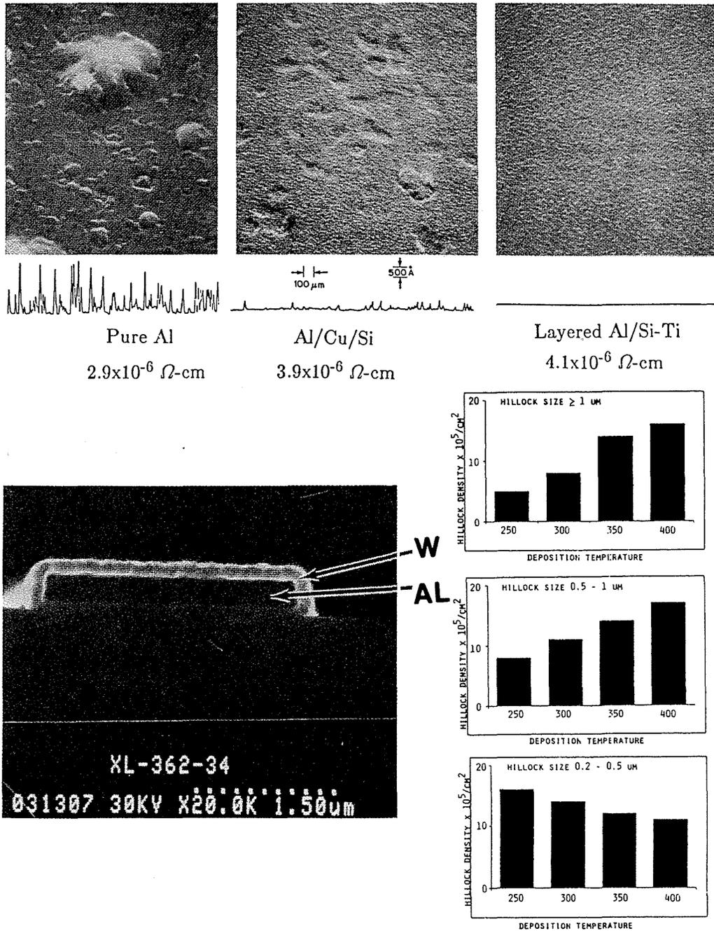
Fig. 4-55 (a) Comparison of hillocks formed in pure Al, Al/Cu/Si, and layered Al/Si-Ti films following an anneal at 450 °C for 30 min.<sup>177</sup> (© 1985 IEEE). (b) CVD W selectively deposited on an Al runner.<sup>179</sup> (© 1986 IEEE). (c) Hillock distribution on cold-sputtered Al after deposition of 0.9-μm SiO<sub>2</sub> at various temperatures. The time at temperature prior to deposition was held constant at one minute.<sup>182</sup> (© 1987 IEEE).
