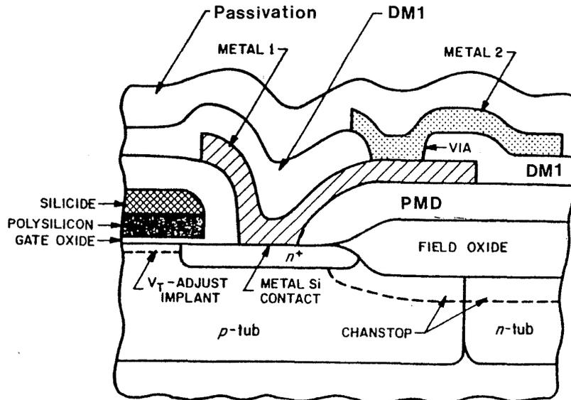
Fig. 4-7 Terminology of double-level-metal interconnects.
