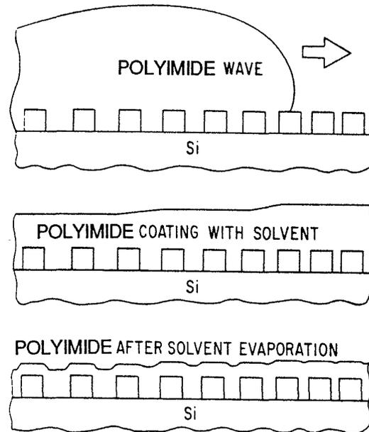
Fig. 4-19 Although the surface of polyimide film is planar when first spun on in liquid form (a) and (b), as the film is cured, solidified and shrunk, the steps on the surface reappear (c), especially at widely spaced features.
