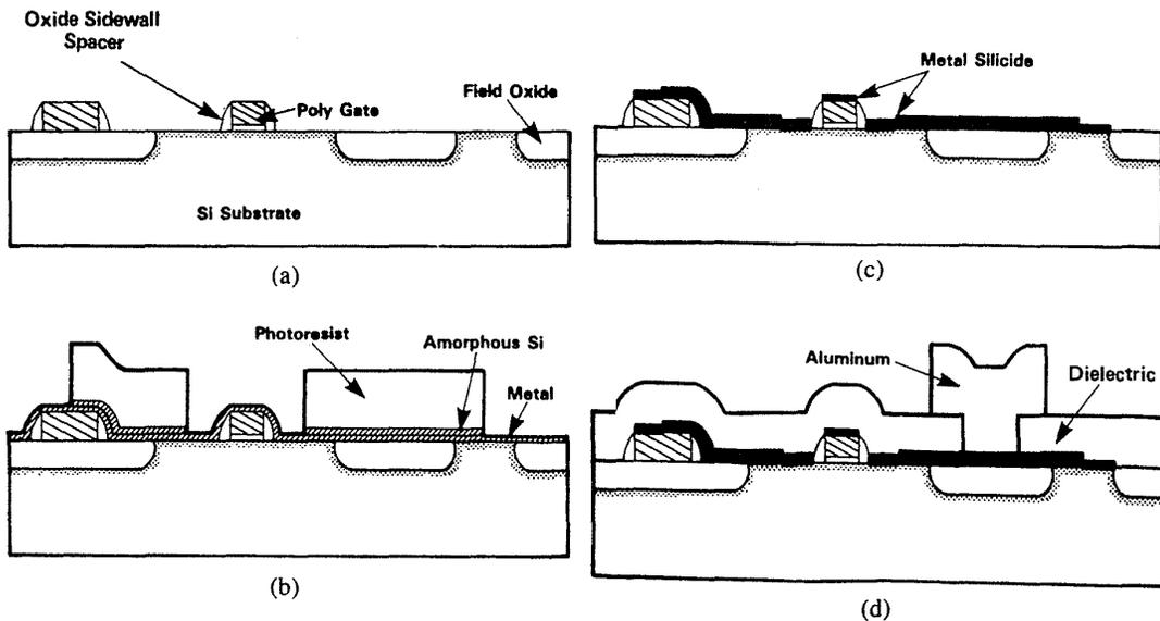
**Fig. 3-52** Fabrication of HPSAC technology. Cross-sectional view after (a) sidewall spacer formation; (b) patterning and etching of amorphous silicon layer; (c) silicide formation; and (d) aluminum alloying.<sup>122</sup> (© 1984 IEEE).
