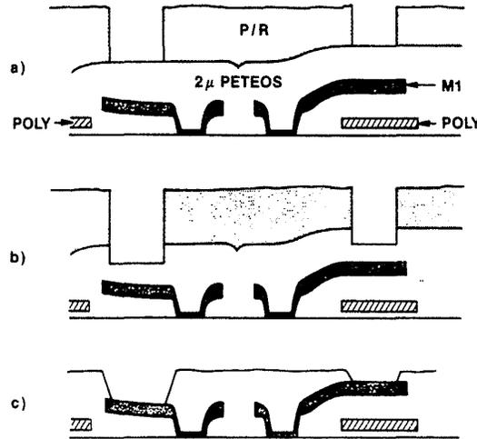
Fig. 4-28 Sequence showing how the etchback and via-sloping processes can be integrated to reduce the overall number of process steps. This paper was originally presented at the Spring 1988 Meeting of The Electrochemical Society, Inc. held in Atlanta, GA.
