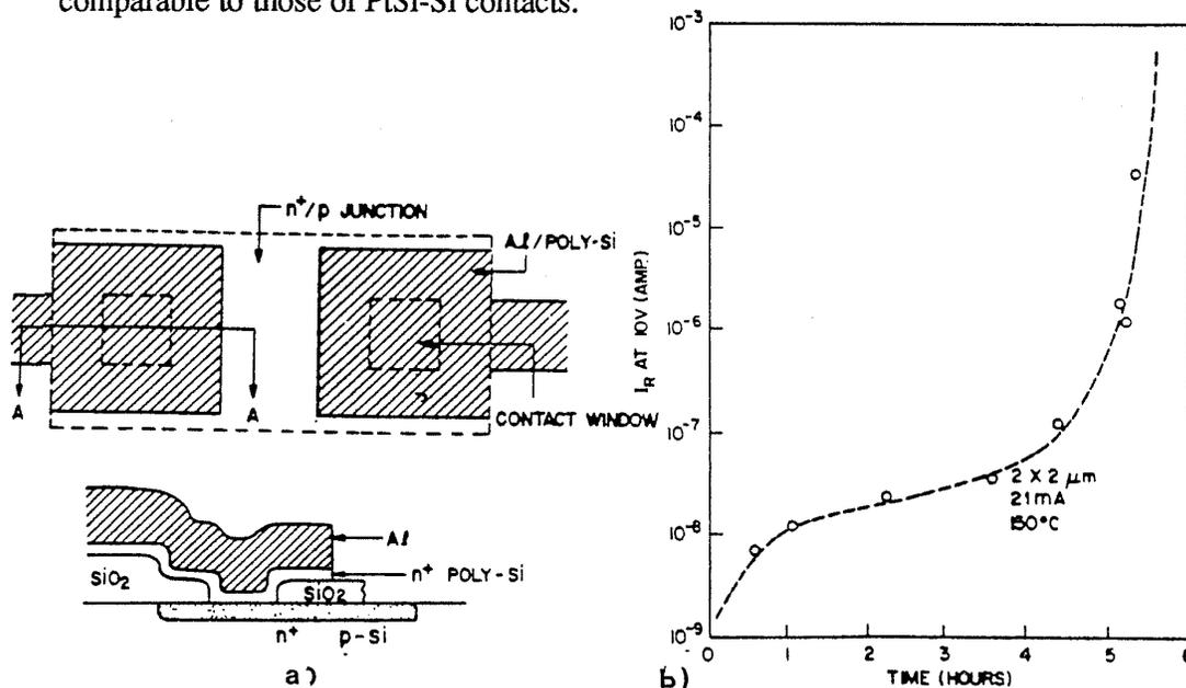
Fig. 3-28 Al-polysilicon-Si contact structure. (a) Layout and cross section. (b) Junction leakage after passing 21 mA at  $150^\circ\text{C}$  through a  $2 \times 2 \mu\text{m}$  contact hole versus time.<sup>55</sup> Copyright 1981. Reprinted with permission of the AIOP.
