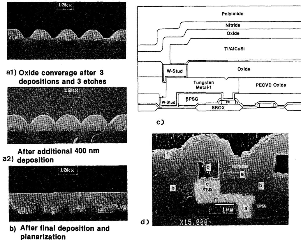
Fig. 4-60 Submicron-CMOS DLM process. (a) and (b) SEM photographs of CVD-oxide gap fill and planarization. (c) Cross section of the completed DLM structure. (d) SEM cross-sectional photograph of this structure.<sup>128</sup> (© 1987 IEEE).
