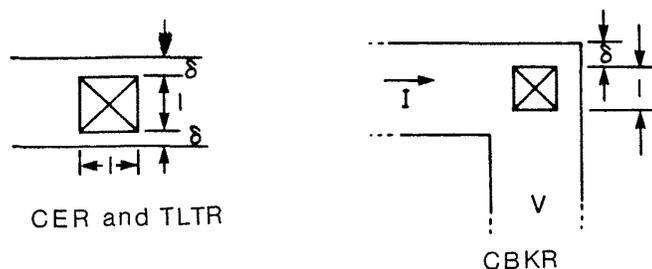
Fig. 3-9 Diffusion region overlap in the three test structures used for measuring contact resistance.<sup>7</sup> (© 1987 IEEE).
