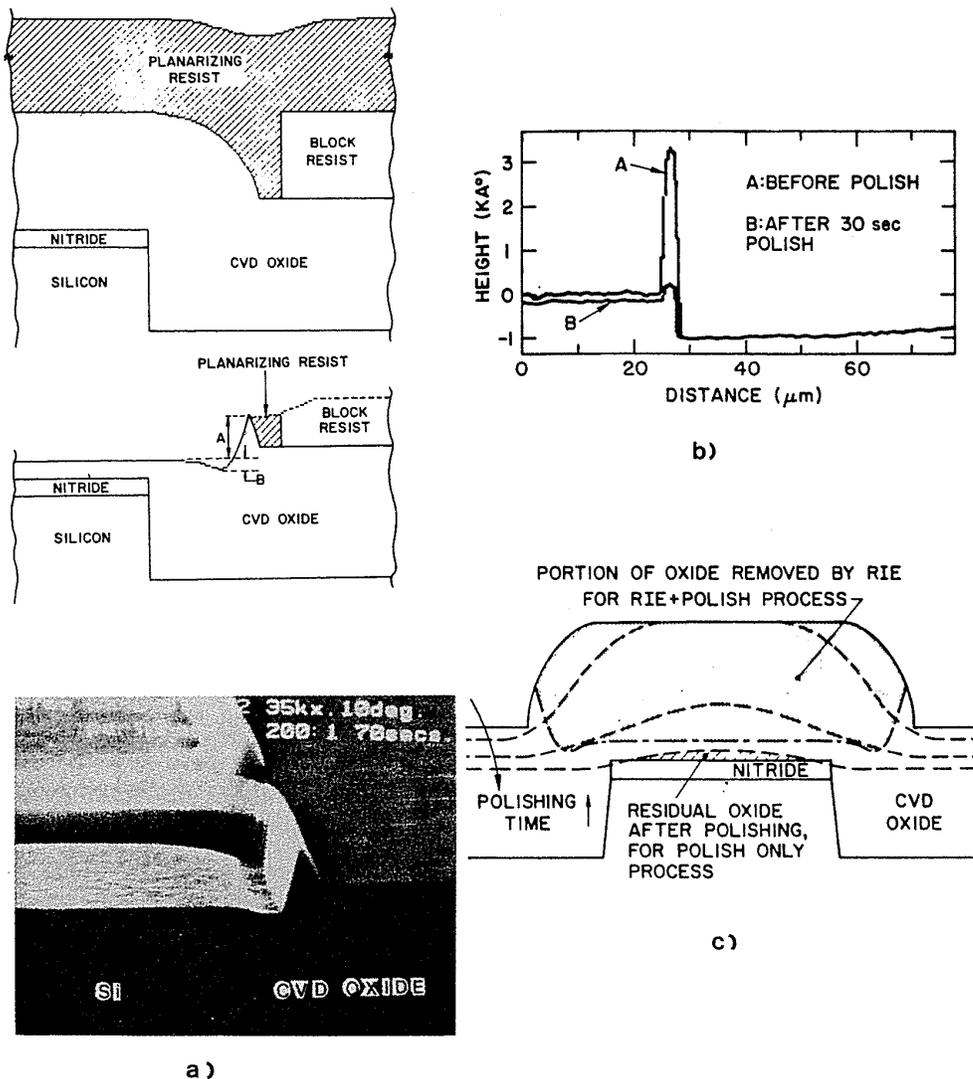
Fig. 4-35 (a) Cross section after selective RIE etchback, showing local oxide spikes that remain after the etchback when the oxide/resist etch-rate ratio > 1. (b) Measured oxide step heights before and after CMP, showing the fast removal rate of such spikes. (c) Schematic drawing showing the fundamental problem of "CMP-only" planarization.<sup>264</sup> (© 1989 IEEE).
