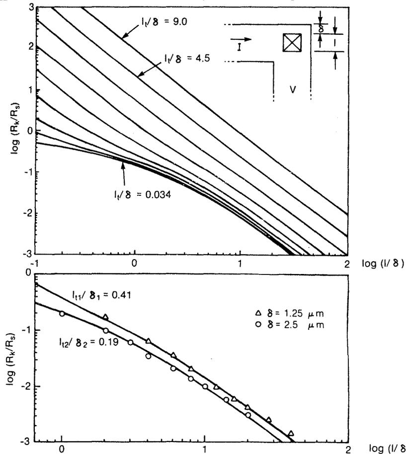
Fig. 3-10 (a) Generalized universal curves for the CBKR. Curves show  $l_t/\delta$  approximately in octave steps. (b) Illustration of the use of the CBKR universal curve to extract  $l_t$  from devices with a different overlap  $\delta$  on the same wafer,  $l_t = 0.5 \mu\text{m}$  for all points.<sup>7</sup> (© 1987 IEEE).
