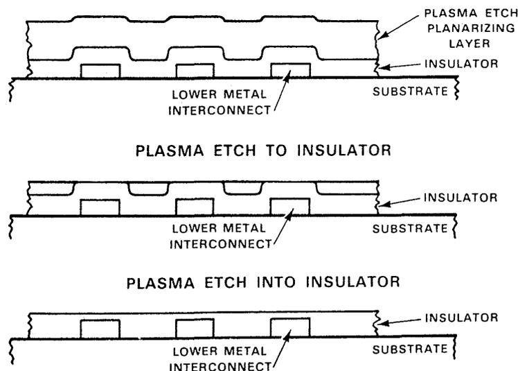
Fig. 4-23 Sequence of steps used in a sacrificial-layer-etchback process for planarization.
