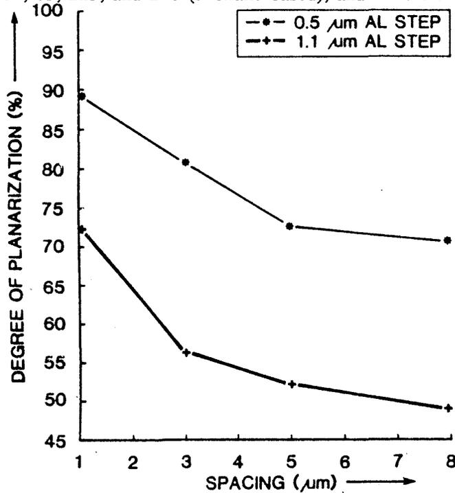
Fig. 4-29 Example of planarization by one type of SOG material as a function of spacing between steps. The underlying oxide step heights are 0.5 and 1.0 μm.<sup>77</sup> (© 1988 IEEE).
