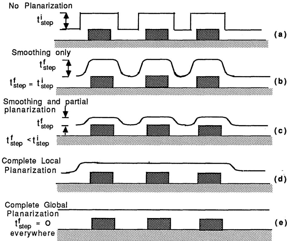
Fig. 4-9 Degrees of dielectric planarization
