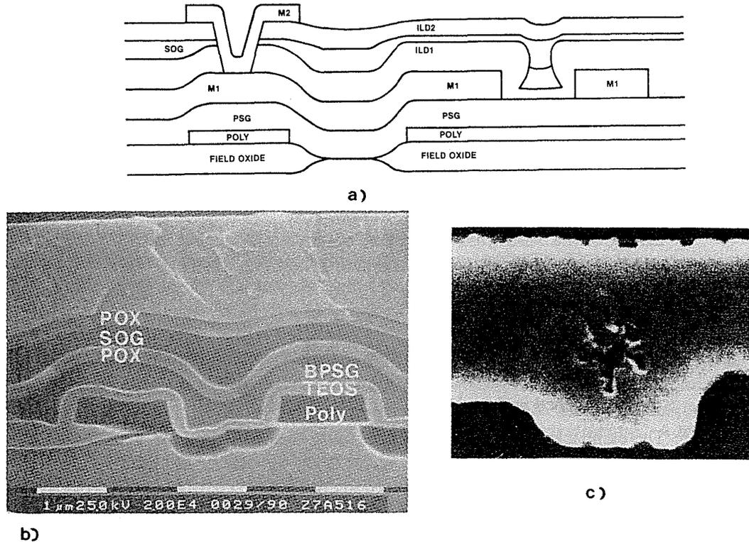
**Fig. 4-33** (a) Drawing of a cross-section of structure formed using the non-etchback SOG process. (b) SEM micrograph of a structure formed with the non-etchback SOG process.<sup>77</sup> (© 1987 IEEE) (c) SEM micrograph of a cross section of a "poisoned via."<sup>93</sup> (© 1987 IEEE).
