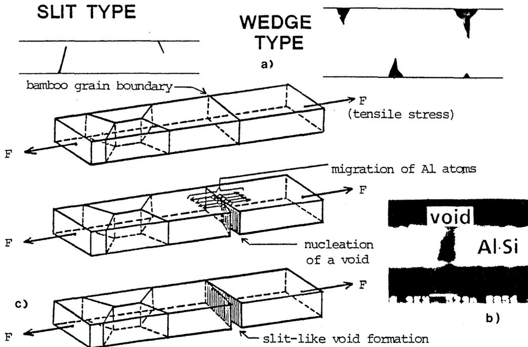
Fig. 4-51 (a) Schematic drawing of stress-induced voids in Al interconnect lines. (b) SEM photo of such a void. (c) Schematics of one proposed formation-mechanism of slit-like voids.<sup>260</sup> (© 1985 IEEE).
