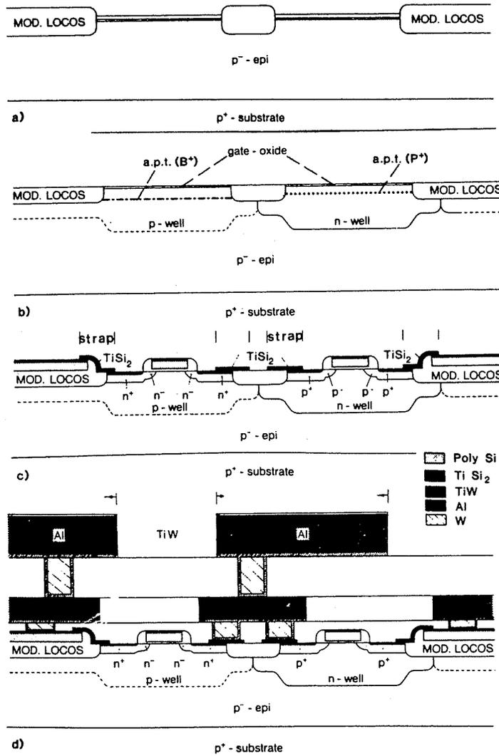
**Fig. 4-59** Schematic cross section of submicron-CMOS DLM technology that uses: a fully planarized isolation structure;  $TiSi_2$  over poly as a local interconnect; selective W as a contact hole plug; and Al:Cu for Metal 1 and Metal 2.<sup>207</sup> (© 1987 IEEE).
