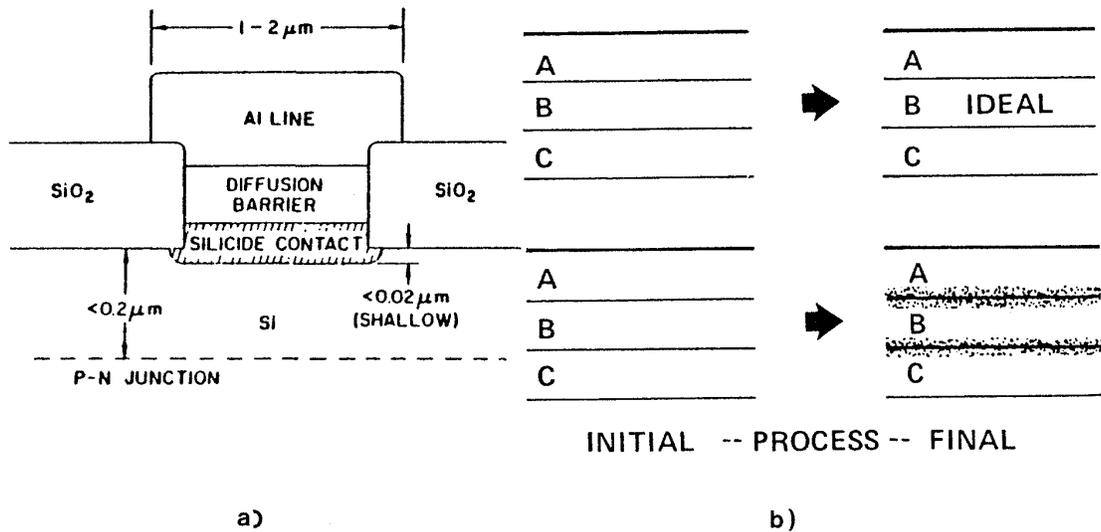
Fig. 3-26 (a) Addition of another layer of material (the diffusion barrier) between the Al and the silicide (or just the Si) to prevent degradation of the contact properties under high temperature processing. (b) Diffusion barrier (material X) reduces intermixing of A and B.
