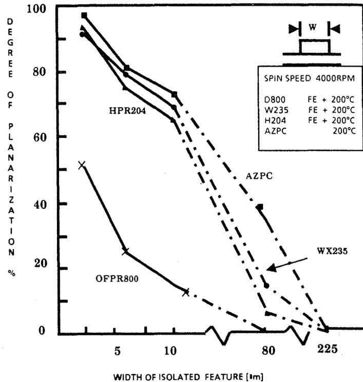
Fig. 4-24 Degree of planarization versus various feature sizes for different polymer films.<sup>64</sup> (© 1987 IEEE).
