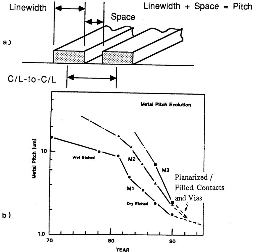
Fig. 4-2 (a) Definition of *metal pitch*. (b) Advanced process integration techniques have enabled the development of multilayer interconnects with tight pitches.<sup>218</sup> This paper was originally presented at the Spring 1989 Meeting of The Electrochemical Society, Inc. held in Los Angeles, CA.
