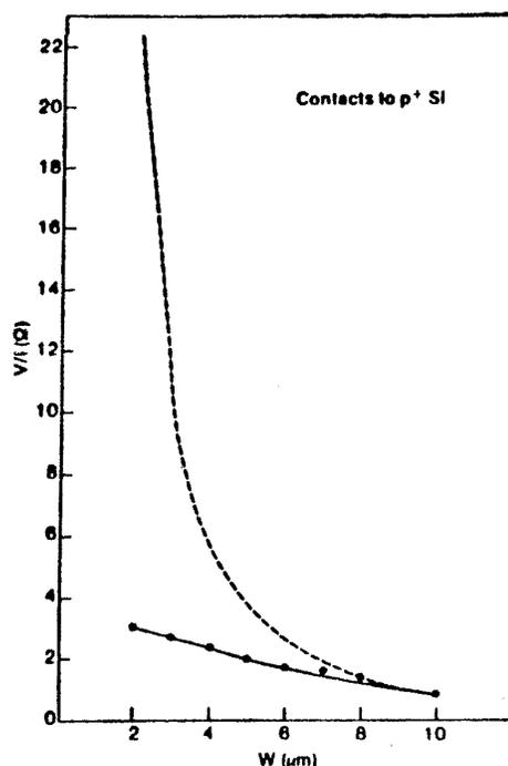
Fig. 3-7 Values of  $R_{CO}$  for small contacts predicted by Eq. 3-4 compared to measured values.<sup>3</sup> Reprinted by permission of the publisher, The Electrochemical Society, Inc.
