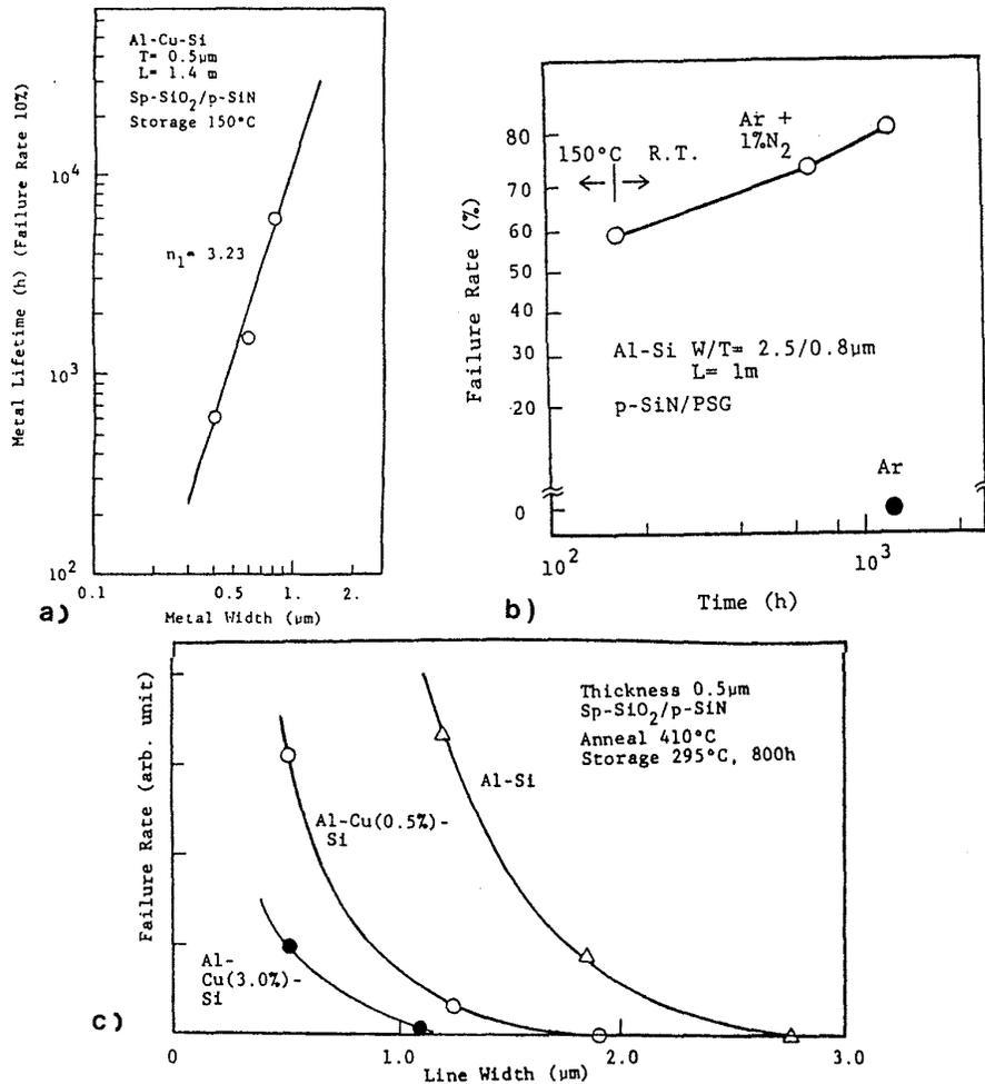
Fig. 4-52 (a) Line width dependence of stress-induced migration of Al:Si:Cu. (b) Stress-induced migration enhanced by N<sub>2</sub> contamination. (c) Dependence of stress-induced migration on the Cu content of the Al films.<sup>168</sup> This paper was originally presented at the Fall 1988 Meeting of The Electrochemical Society, Inc. held in Chicago, IL.
