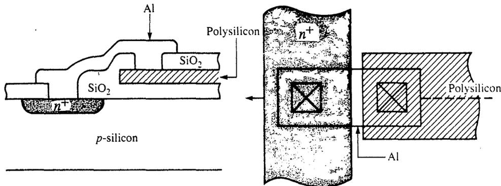
Fig. 3-48 Aluminum film link for connecting polysilicon and the silicon substrate with an intervening space. From R. C. Jaeger, *Introduction to Microelectronic Fabrication*. Copyright, 1988, Addison-Wesley. Reprinted with permission.
