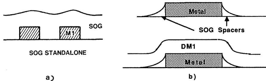
Fig. 4-31 (a) SOG standalone film. (b) Spin on SOG over underlying metal; etchback to leave SOG spacers; deposit DM1 oxide over this structure.
