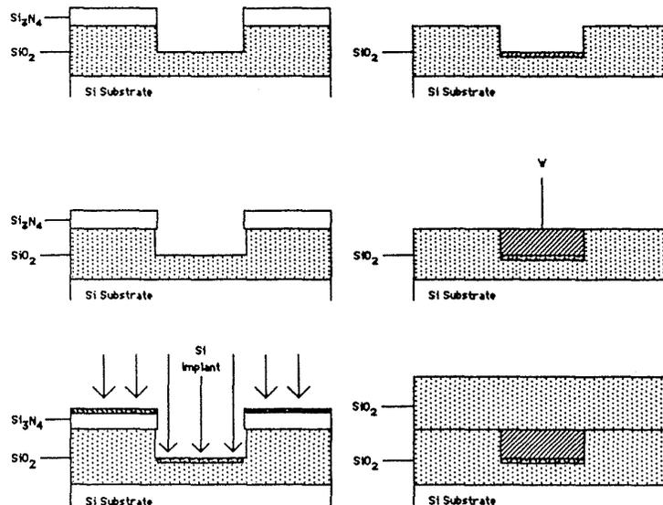
Fig. 4-49 Process flow for planar *W* interconnect technology (WIT).<sup>158</sup> (© 1988 IEEE).
