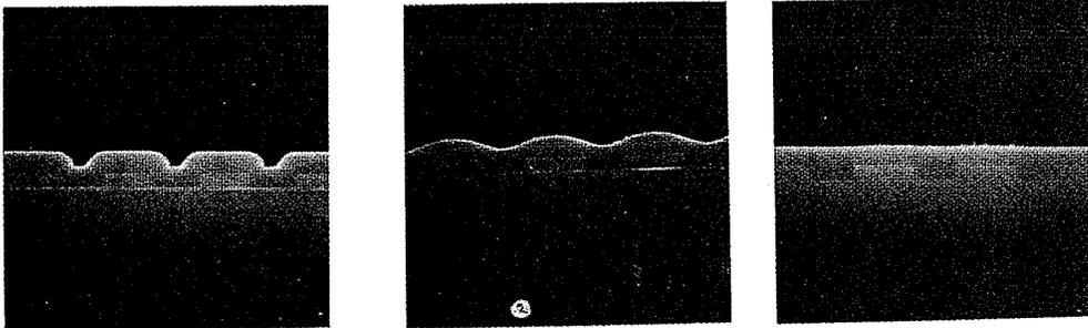
Fig. 4-15 Planarization of the PMD layer (BPSG) by thermal flow.<sup>28</sup> Reprinted with permission of Semiconductor International.
