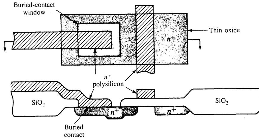
Fig. 3-50 Cross section of a buried-contact structure. From R. C. Jaeger, *Introduction to Microelectronic Fabrication*. Copyright, 1988, Addison-Wesley. Reprinted with permission.
