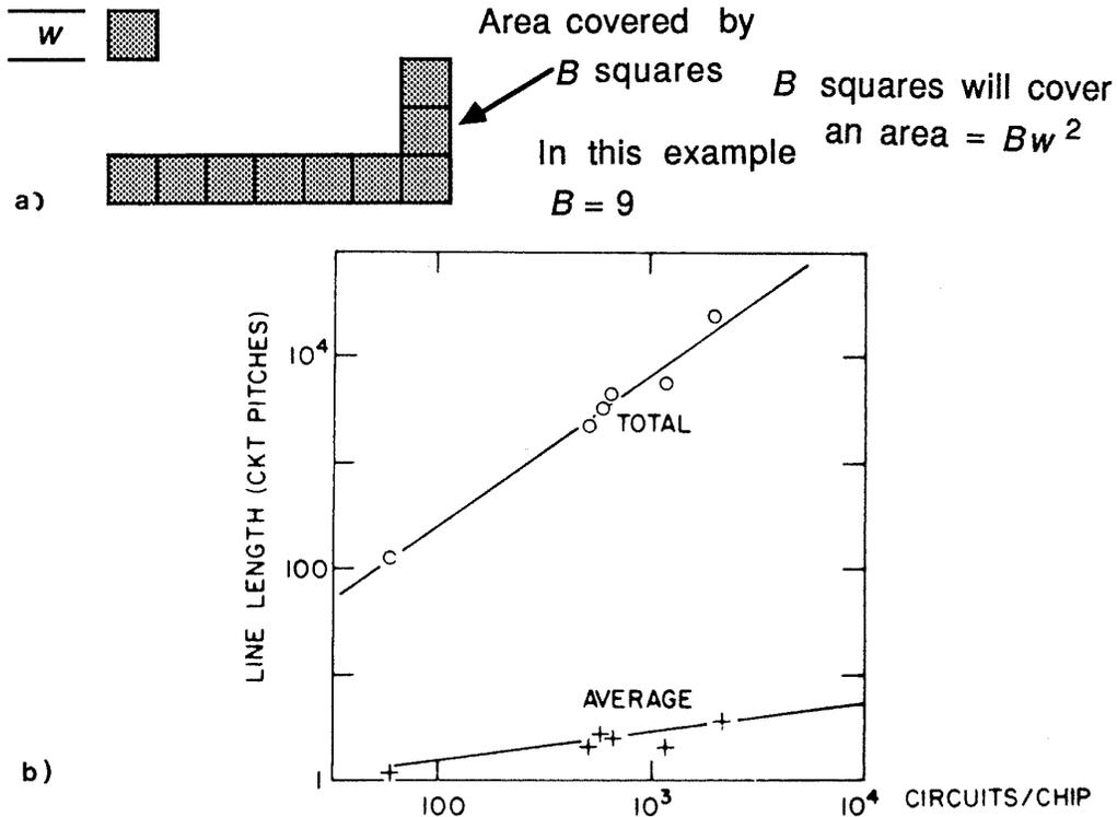
Fig. 4-3 (a) The area of a chip covered with  $B$  squares of metal whose sides are  $w$  wide, is  $Bw^2$ . (b) The average length of interconnect and the total wire length on a logic chip as a function of device density. The lengths are measured in circuit pitches, i.e., the square root of the area per circuit.<sup>1</sup> (© 1981 IEEE).
