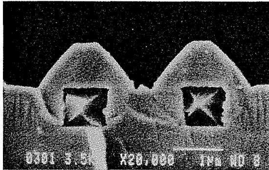
Fig. 4-22 At the conclusion of a CVD/Etch process, the surface topography over narrow lines will have a pyramid structure.<sup>58</sup> (© 1987 IEEE).
