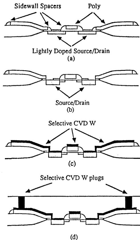
**Fig. 3-56** Processing sequence of selective CVD W local interconnect technology. Cross sectional view after (a) sidewall spacer formation, (b) selective removal of sidewall spacer of local interconnect and source/drain formation, (c) selective CVD W deposition, and (d) selective CVD W plug filling.<sup>128</sup> (© 1988 IEEE).
