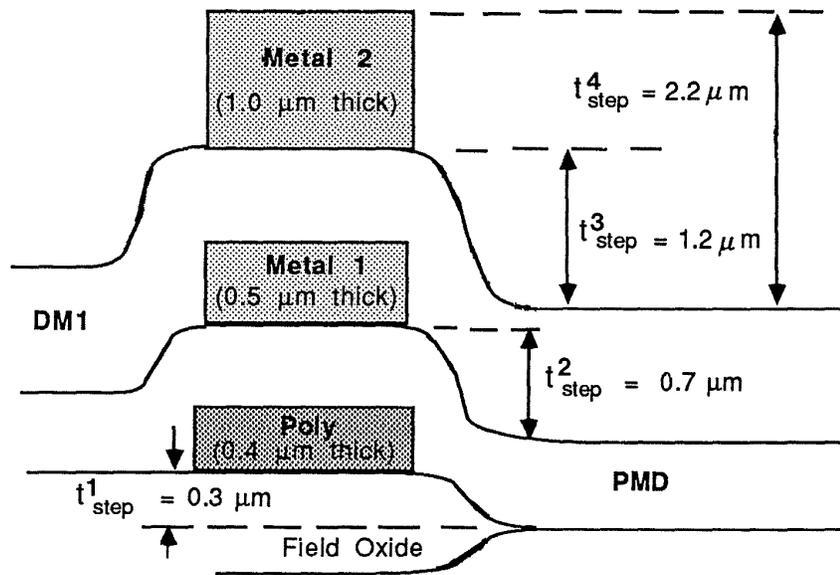
**Fig. 4-10** As the number of levels in an interconnect technology is increased, the stacking of additional layers on top of one another produces steps of progressively greater heights.
