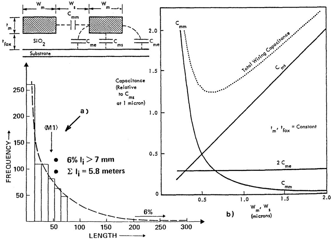
Fig. 4-5 (a) Example of lead length distribution of metal interconnects on an IC having a single level of metal.<sup>4</sup> Reprinted with permission of Electronics. (b) Variation of components of interconnect capacitance with design rules. The various components are defined in the adjacent figure.<sup>5</sup> (© 1982 IEEE).
