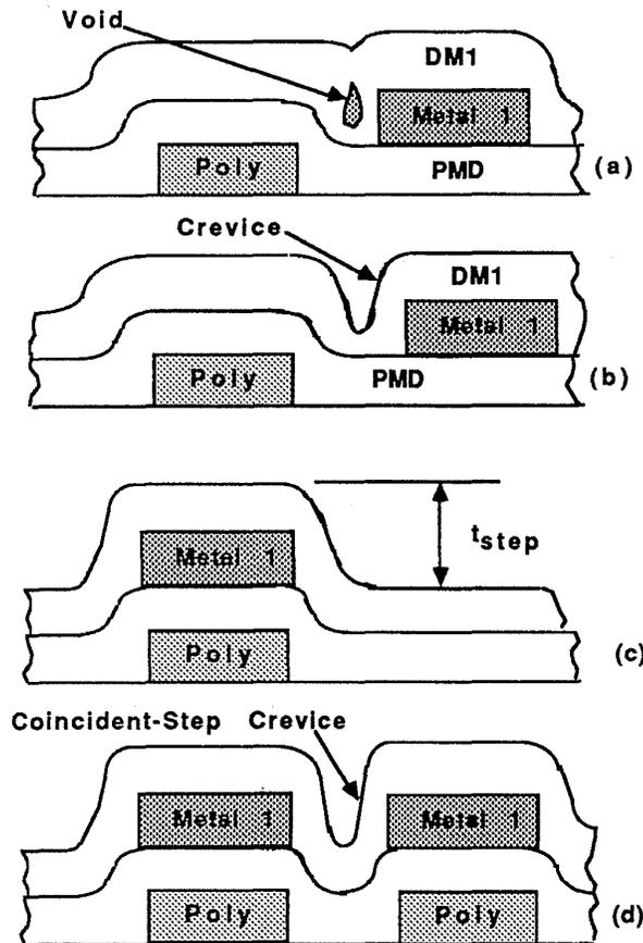
Fig. 4-14 Conditions associated with the relative spacing of polysilicon and Metal 1 that lead to layout design rules of these layers.
