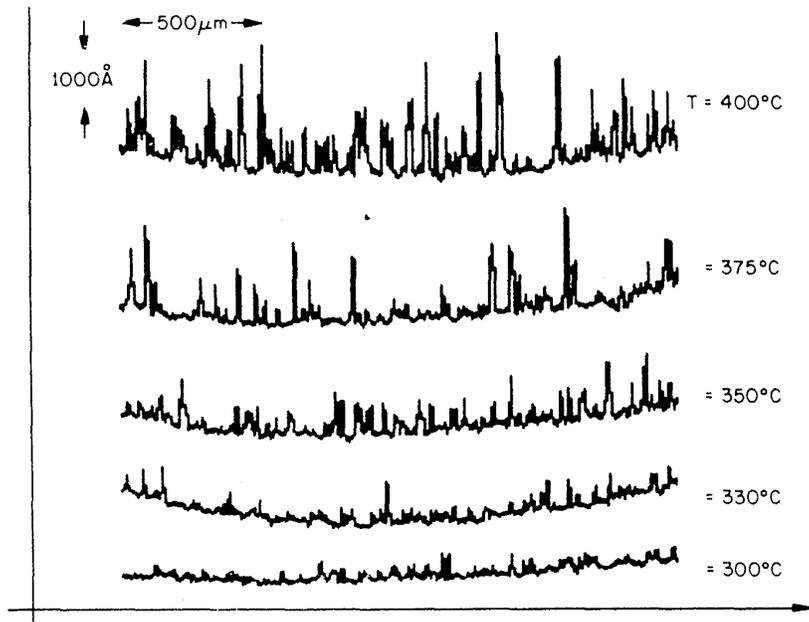
Fig. 4-53 (c) Hillock formation as a function of deposition temperature.<sup>172</sup> (© 1987 IEEE).
