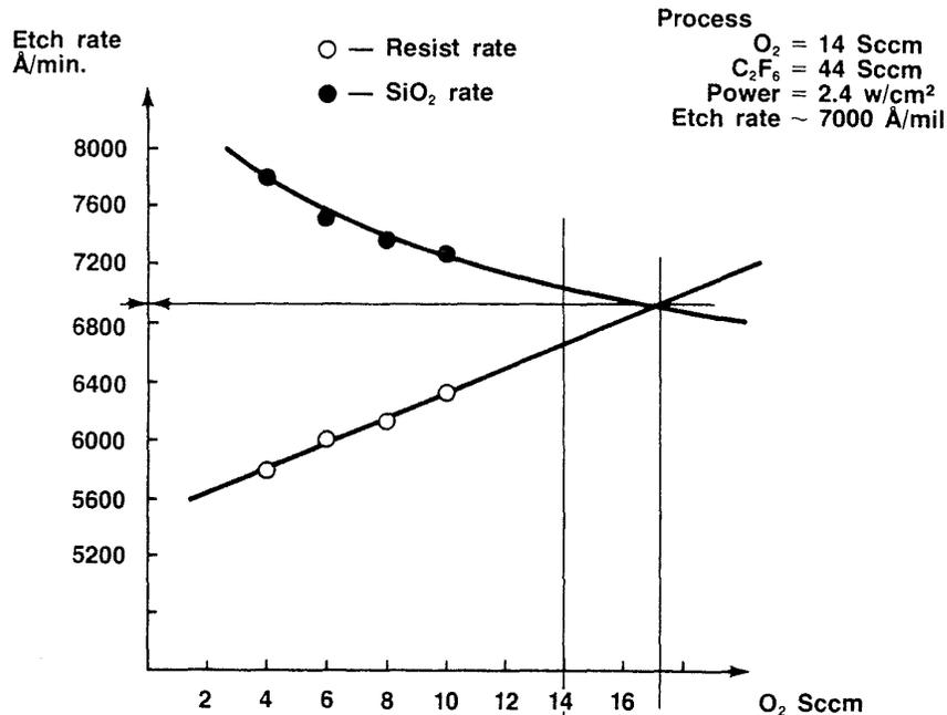
Fig. 4-25 Example of how the etch rates of resist and SiO<sub>2</sub> can be equalized by varying the gas mixture used in the plasma-etching process. Courtesy MRC, Inc.
