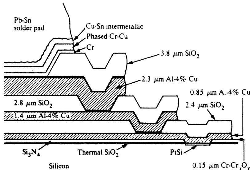
Fig. 4-61 Schematic of an early three-level-metal interconnect structure.<sup>210</sup> Copyright 1982 by International Business Machines Corporation. Reprinted with permission.
