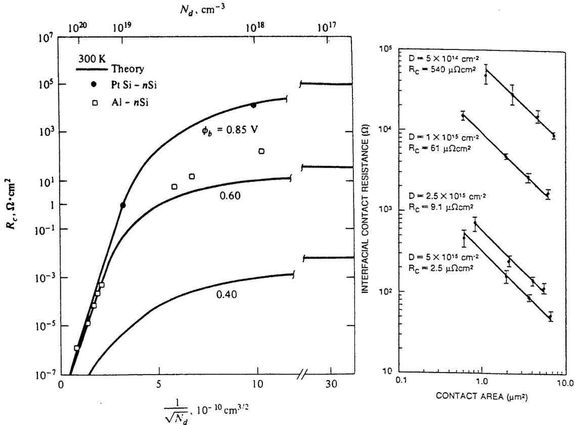
Fig. 3-5 (a) Theoretical and experimental values of specific contact resistance.<sup>1</sup> (© 1971 Solid State Electronics). (b) Specific contact resistivity vs. implant dose.<sup>2</sup> (© 1985 IEEE).
