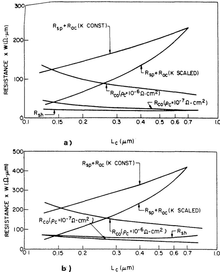
Fig. 3-37 The contributions of each resistance component as a function of channel length,  $L_c$ , for (a) *n*-channel and (b) *p*-channel MOSFETs.<sup>85</sup> (© 1987 IEEE).
