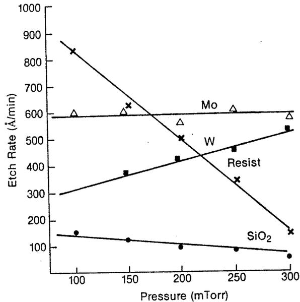
Fig. 4-41 Etch conditions used for W plug formation using photoresist planarization. Etch parameters are: flow – 60 sccm, 75% O<sub>2</sub> in CCl<sub>2</sub>F<sub>2</sub>/O<sub>2</sub>; and power – 300 W (0.25 W cm<sup>2</sup>); and a carbon cathode cover in the reactive ion etcher.<sup>137</sup> (© 1986 IEEE).
