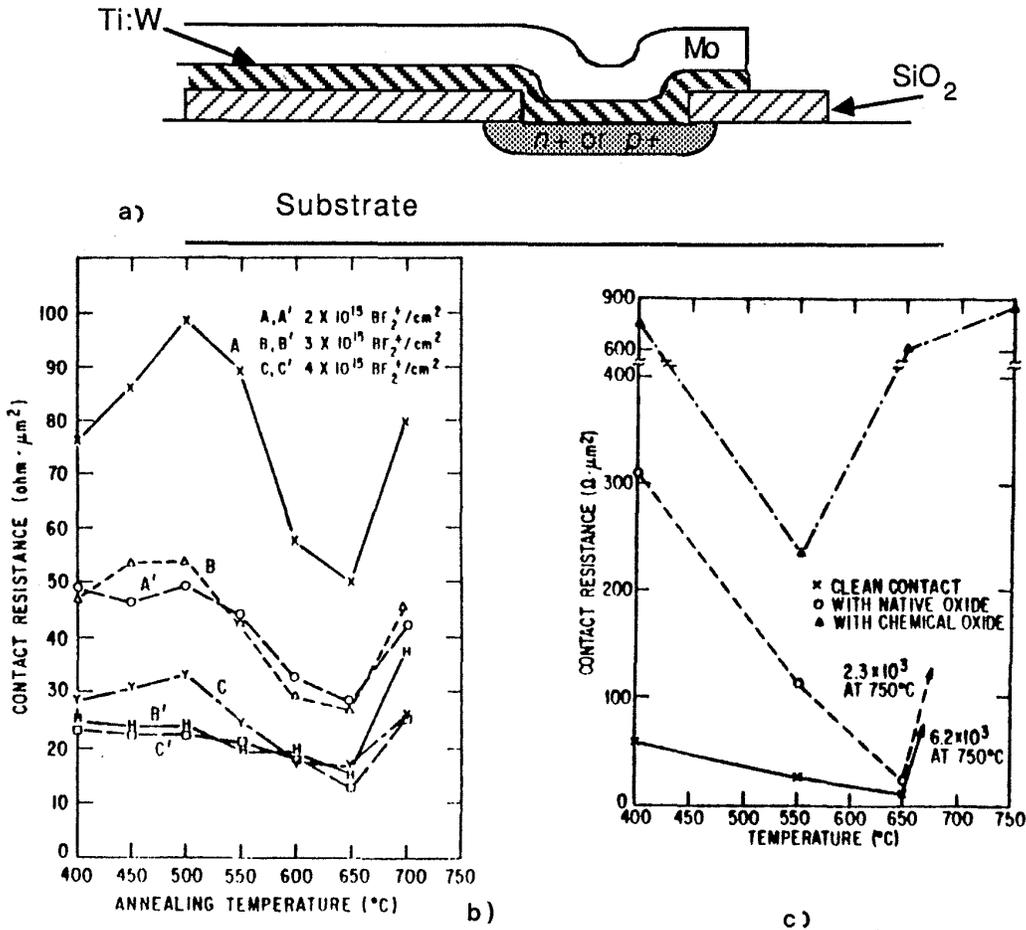
Fig. 3-31 Mo-Ti:W-Si contacts. (a) Structure cross section. (b) Effect of isochronal annealing on the  $p^+$  contact resistance versus  $\text{BF}_2^+$  implant dose. (c) Contact resistance change to  $n^+$  Si as a function of isochronal annealing temperature with and without interface oxide.<sup>82</sup> Reprinted by permission of the publisher, The Electrochemical Society, Inc.
