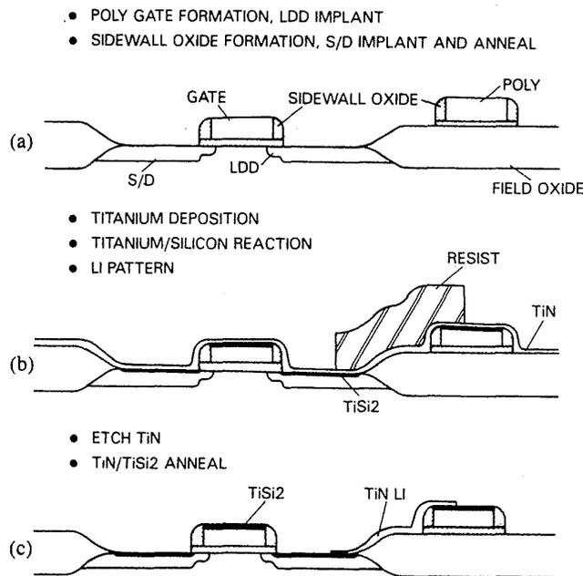
Fig. 3-54 Self-aligned  $\text{TiSi}_2$  process showing the TiN LI patterning step.<sup>124</sup> (© 1987 IEEE).
