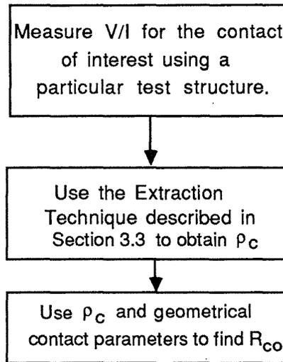
Fig. 3-6 Flow chart that illustrates how to obtain accurate values of  $R_{CO}$  in an actual contact.
