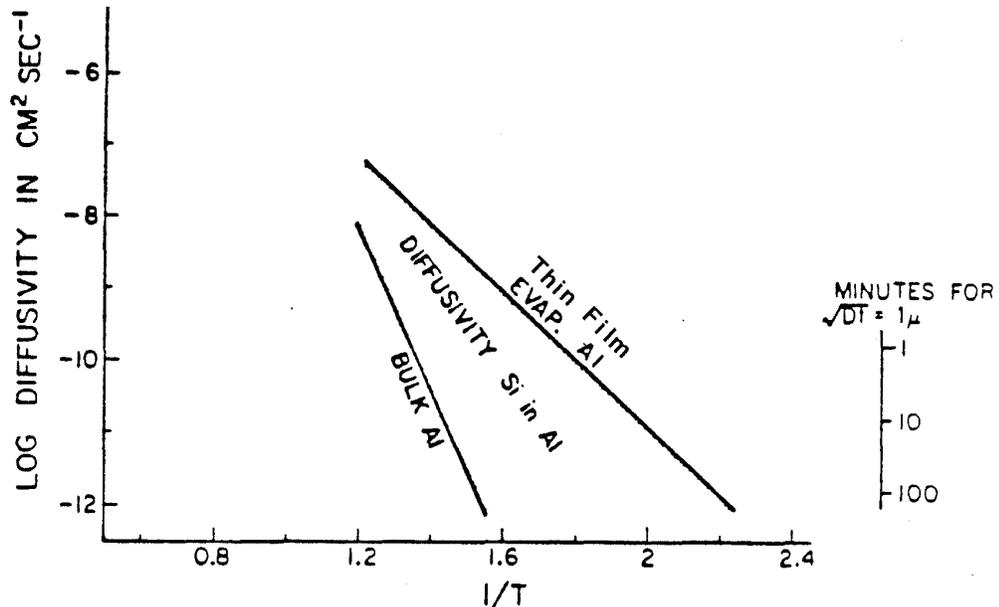
Fig. 3-20 Diffusivity of silicon in bulk and thin film aluminum.<sup>32</sup> Copyright 1974. Reprinted with permission of the AIOP.
