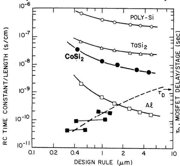
**Fig. 4-4** RC time constant per unit length for several conductive materials as a function of feature size. Also shown is delay per stage of NMOS ring oscillators as a function of feature size. The RC time constant is calculated assuming a field oxide thickness of  $1 \mu\text{m}$ .<sup>258</sup> Copyright 1981 AIOP. Reprinted with permission.
