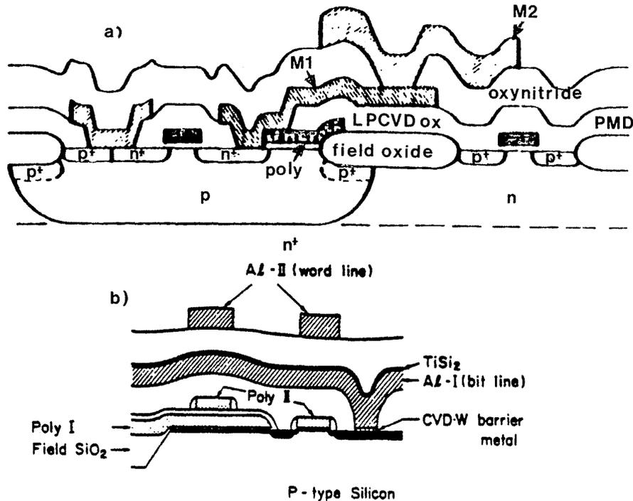
Fig. 4-57 (a) Example of a double-level-metal CMOS process with no planarization.<sup>197</sup> (© 1984 IEEE). (b) DLM process with a CVD W barrier metal and TiSi<sub>2</sub> hillock-suppression layer on top of the Metal-1 Al layer.<sup>200</sup> (© 1984 IEEE).
