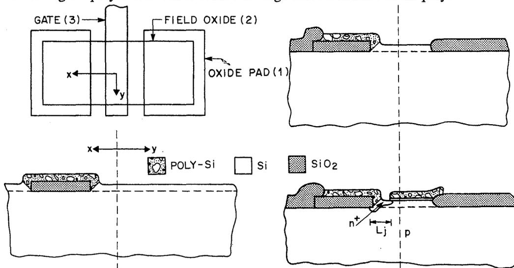
Fig. 3-42 The key process steps of the BOMOS self-aligned contact approach.<sup>164</sup> (© 1987 IEEE).
