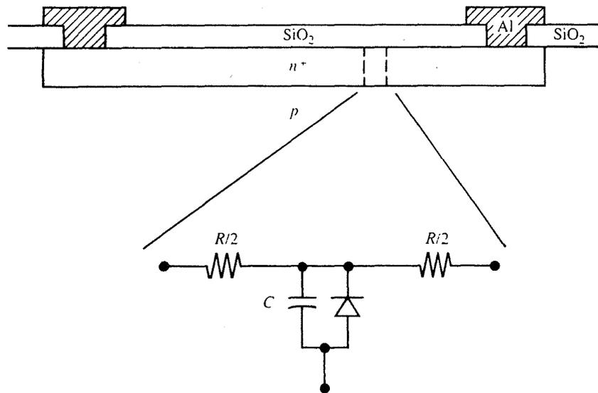
Fig. 4-1 A lumped circuit model for a small section of an  $n^+$  diffusion. The RC delay limits the use of diffusions for high-speed signal distribution. From R. C. Jaeger, *Introduction to Microelectronic Fabrication*. Copyright, 1988, Addison-Wesley. Reprinted with permission.
