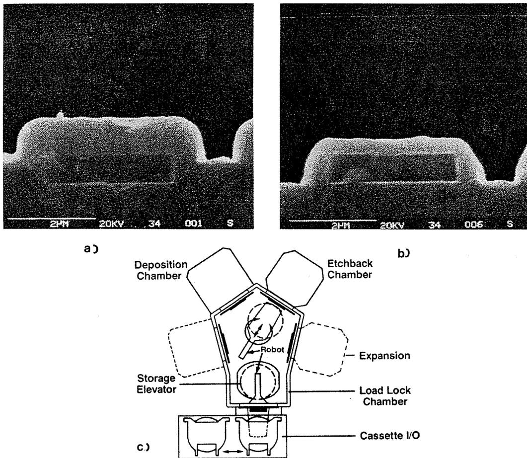
Fig. 4-21 CVD SiO<sub>2</sub> and in situ etchback. (a) Photograph of an as deposited PECVD oxide over vertical sidewalled Metal 1 lines. (b) Shape of PECVD oxide after reactive ion etching using energetic ion bombardment.<sup>54</sup> (© 1987 IEEE). (c) Example of a multi-chamber tool that can perform deposition in one chamber and etching in another. Courtesy of Applied Materials.
