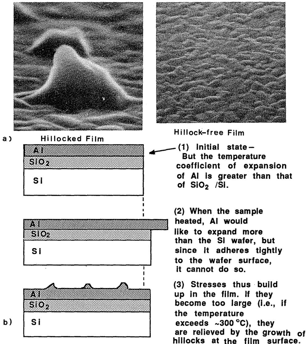
Fig. 4-53 (a) SEM photo of hillock and hillock-free Al thin film. (b) Schematic drawing of how thermal stress causes hillock growth in Al thin films on a Si wafer.
