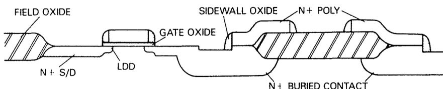
**Fig. 3-51** Limitations of buried contacts: (1) Phosphorus outdiffusion limits device isolation and buried-contact-to-gate design-rule scaling. (2) The use of *n*-type polysilicon limits buried contacts in CMOS to *n*-channel transistors only.<sup>124</sup> (© 1987 IEEE).
