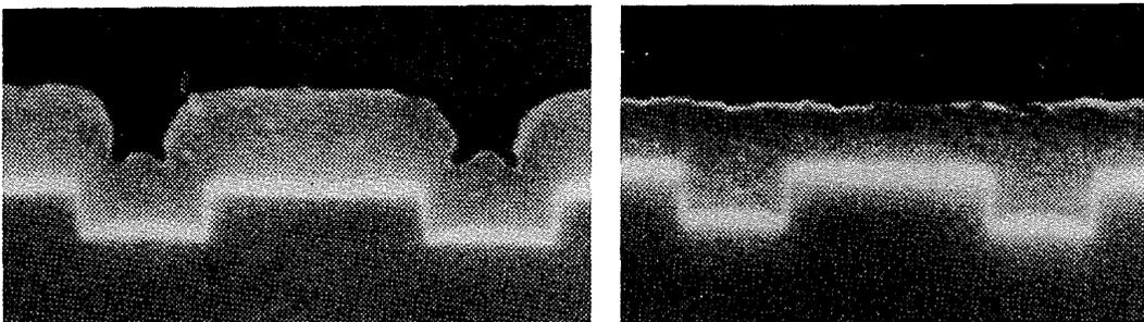
Fig. 4-45 SEM photos of an Al film before and after laser planarization.<sup>210</sup> Reprinted with permission of Solid State Technology.
