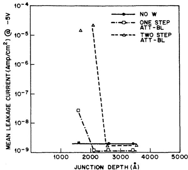
Fig. 3-30 Comparison of mean leakage current density vs.  $n^+$  (As/P) junction depth in Si for contacts fabricated with no W and for W deposited with the hydrogen reduction process.<sup>70</sup> This paper was originally presented at the Spring 1988 Meeting of The Electrochemical Society, Inc. held in Atlanta, GA.
