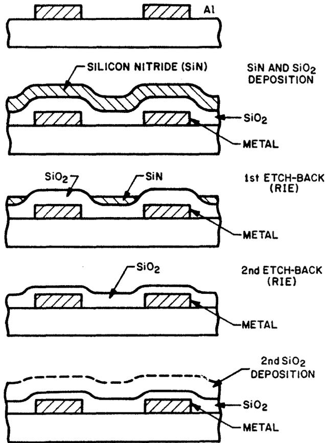
Fig. 4-27 Example of a sacrificial-etchback process that uses SiN as the sacrificial film.<sup>75</sup>
