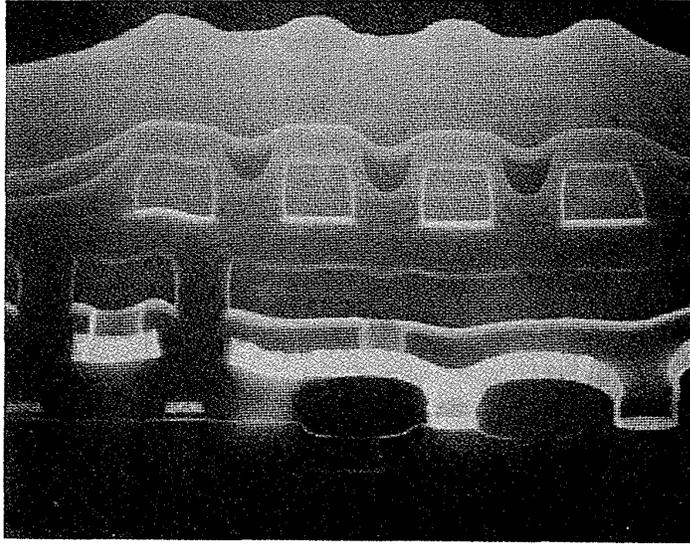
Fig. 4-63 SEM photograph of another completed four-level-metal interconnection structure.<sup>236</sup> (© 1988 IEEE).
