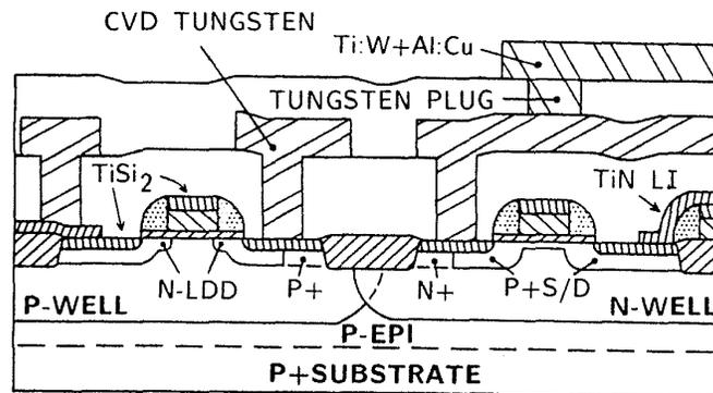
Fig. 4-58 Schematic cross section of a 0.8- $\mu\text{m}$  CMOS DLM process.<sup>205</sup> (© 1987 IEEE).
