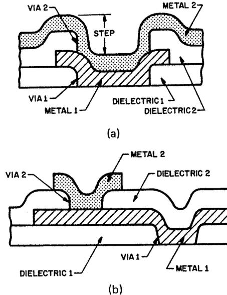
Fig. 4-37 Contact schemes: (a) stacked vias; and (b) staggered vias. From A. G. Sabnis, in G. S. Gildeenblat and S. S. Cohen, Eds., *VLSI Electronics: Microstructure Science, Vol. 15, Metallization*, Chap. 7. Copyright 1987, Academic Press. Reprinted with permission.
