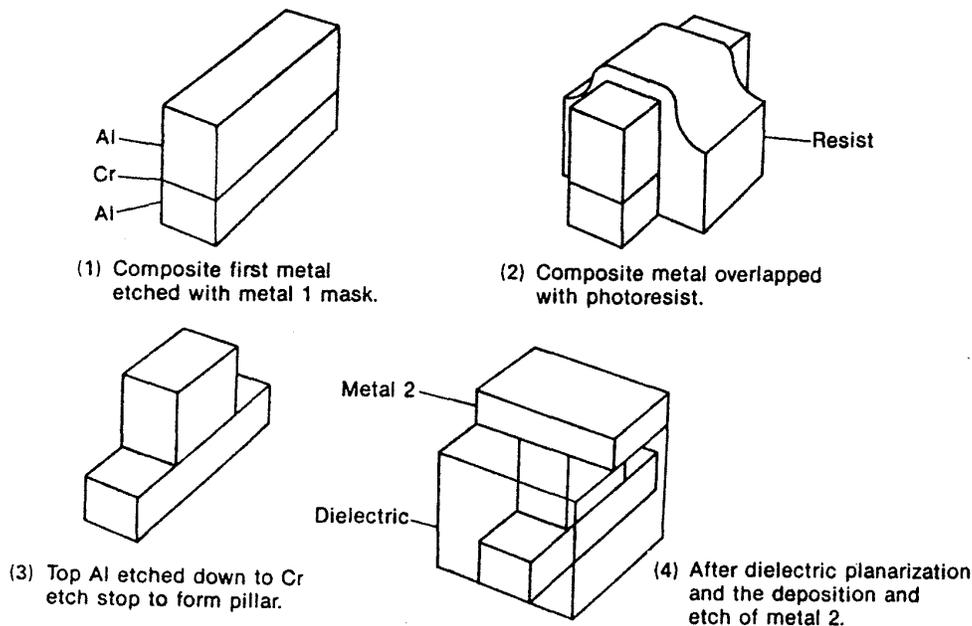
Fig. 4-47 Sequence used to produce Al/Cr/Al pillars using photoresist overlap method.<sup>251</sup> (© 1984 IEEE).
