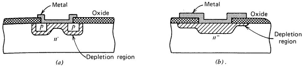
**Fig. 3-34** Special processing techniques improve the performance of Schottky diodes. (a) The diffused guard ring leads to a uniform electric field and eliminates breakdown at the junction edge. (b) The field plate is an alternative means for achieving the same effect. From R. S. Muller and T. I. Kamins, 2nd Ed., *Device Electronics for Integrated Circuits*. Copyright 1986, John Wiley & Sons. Reprinted with permission.
