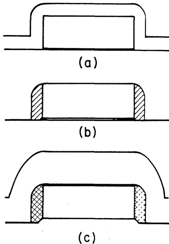
**Fig. 4-18** Spacer formation: (a) CVD deposition over a polysilicon line; (b) spacer formation by RIE; (c) spacer structure covered with CVD oxide.
