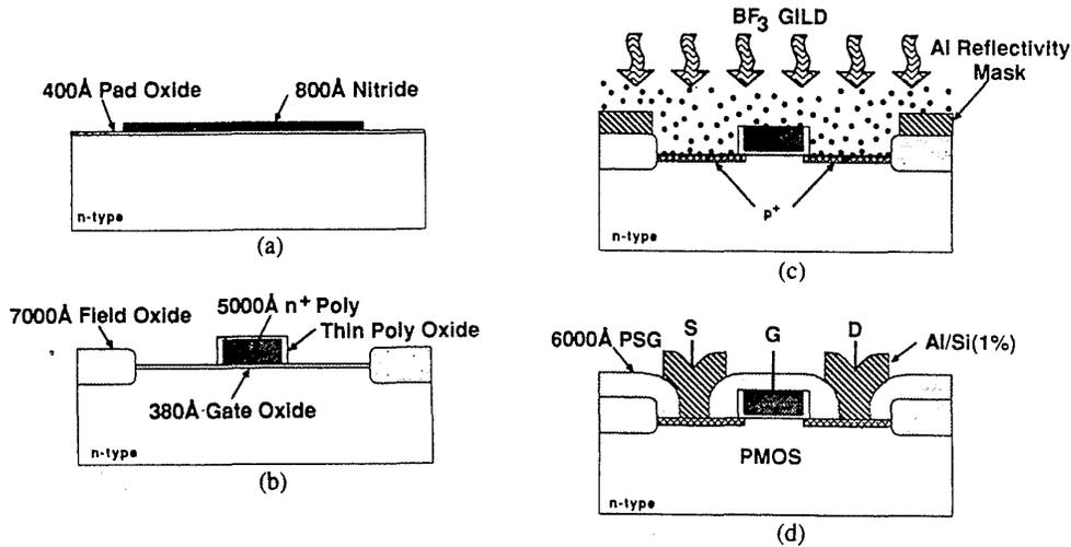
Fig. 3-46 Key steps in the GILD PMOS process: (a) active area definition, (b) after poly deposition,  $n^+$  doping, patterning, and oxidation, (c) GILD laser doping step for  $p^+$  source/drain formation, and (d) after PSG and Al/Si (1%) deposition and etching.<sup>121</sup> (© 1988 IEEE).
