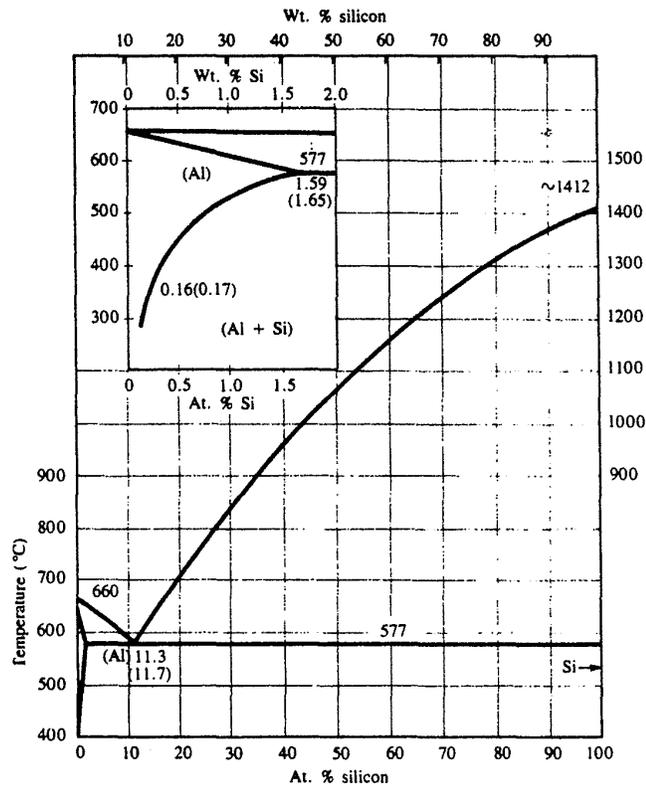
**Fig. 3-19** Phase diagram of the aluminum-silicon system. The silicon-aluminum eutectic point occurs at a temperature of 577 °C. At contact-alloying temperatures between 450 and 500 °C, aluminum will absorb from 0.5 to 1% silicon. Copyright 1958, McGraw-Hill Book Company, with permission from ref. [161].
