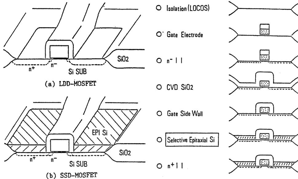
Fig. 3-45 Schematic diagram of (a) an LDD-MOSFET. (b) a stacked-source-drain (SSD) MOSFET using selective epitaxy. (c) Fabrication process flow of an SSD-MOSFET.<sup>118</sup> This paper was originally presented at the Spring 1988 Meeting of The Electrochemical Society, Inc. held in Atlanta, GA.
