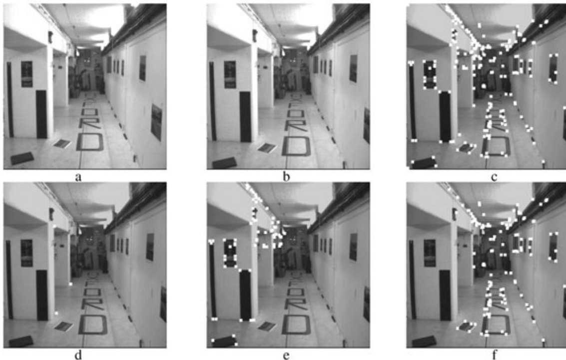
Fig. 13.10. Binary space partition. (a) (b) Left and right images. (c) Points whose correspondence is known. (d) A triplet of points selected from (c). This triplet defines a plane. The points in (c) can then be classified according to their side of the plane. (e) Points on one side. (f) Points on the other side.
