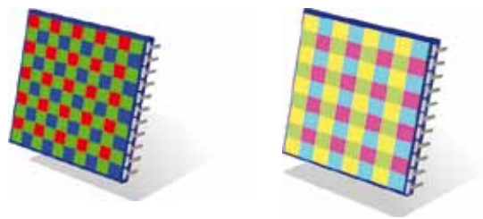
Figure 2. Bayer array color filter (left) and CMYG color filter array (right)
