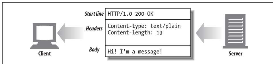
Figure 3-3. Three parts of an HTTP message
