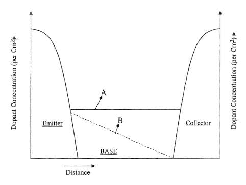
Figure 1 is labeled "Prior Art" and shows a plot of dopant concentration versus distance. Ex. 1001, Fig. 1. According to the '842 patent, Figure 1 "illustrates the relative doping profiles of emitter, base and collector for the two most popular bipolar junction transistors: namely, uniform base ('A') and graded base ('B')." *Id.* at 2:35–38.
