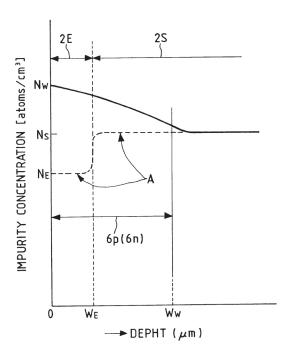
Figure 17 is a plot of impurity concentration as a function of depth in a semiconductor integrated circuit device, which shows "the p-well 6p and n-well 6n have their impurity concentrations gradually lowered in the depthwise direction from the principal surface (having an impurity concentration NW) of the epitaxial layer 2E." Ex. 1007, 5:41–45, 15:62–16:40.
