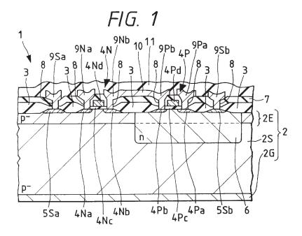
Figure 1 depicts "an essential portion of a semiconductor integrated circuit device" that includes semiconductor substrate body 2S, epitaxial layer 2E, and gettering layer 2G. *Id.* at 6:42–49, 6:51–56, Fig. 1. Substrate body 2S and epitaxial layer 2E are doped with a p-type impurity in equal
