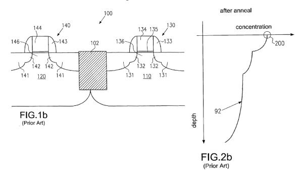
Wieczorek Figure 1b shows a conventional semiconductor device at an early manufacturing stage, including shallow trench isolation 102 separating N-
