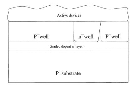
Figure 5A illustrates a cross section of a CMOS silicon substrate with two wells and an underlying layer using embodiments of the invention. *Id.* at 2:54–56. Figure 5A is labeled "[a] CMOS Substrate for digital, mixed[] signal, and sen[s]or[] IC's." Ex. 1001, Fig. 5A. The figure illustrates "a CMOS silicon substrate with two wells and an underlying layer," which is labeled "Graded dopant n<sup>-</sup>layer." *Id.* at 2:54–58, Fig. 5A.
