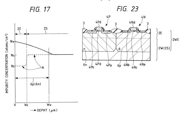
Figure 17 is a plot of impurity concentration as a function of depth in a semiconductor integrated circuit device, which shows "the p-well 6p and n-well 6n have their impurity concentrations gradually lowered in the depthwise direction from the principal surface (having an impurity
