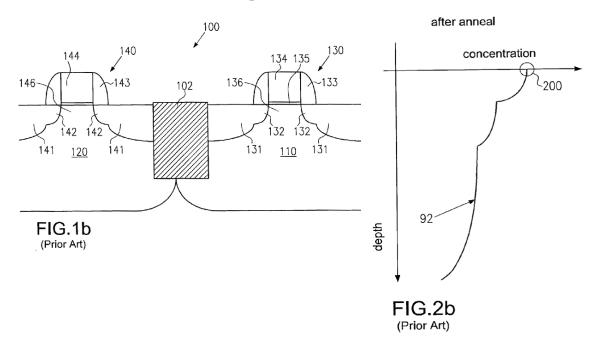
Wieczorek Figure 1b shows a conventional semiconductor device at an intermediate manufacturing stage, including shallow trench isolation 102 separating N-well structure 120 from P-well structure 110. Ex. 1006 ¶¶ 7, 20. The device includes P-channel transistor 140 with source and drain
