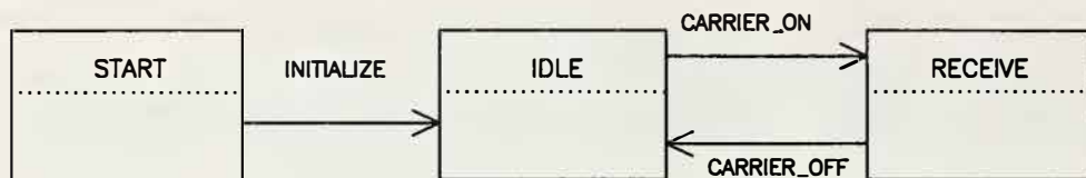
Fig C2 Receive Component State Diagram
