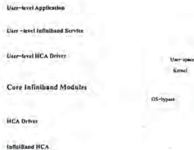
Figure 2. Architectural overview of OpenIB Gen2 stack
