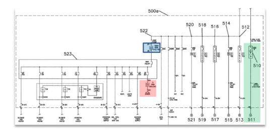
Ex. 1006 Fig. 4. The other electrical connection feeds "blender unit including a slurry power unit VFD 510 for operating a blurry power unit motor 511 (annotated
