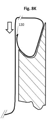
Figure 8K shows that after a series of steps (Figures 8E–8J), thermoplastic article 100 is ultimately urged into ram 300 (identified in Figures 8E, 8H) in the direction indicated by the open arrow to produce a shaped deflectable flange 160 that includes peripheral flange 120 at the peripheral end of spacer 140. *Id.* at 10:56–61. The '624 patent discloses that shaped articles can be "in the form of a rounded rectangular tray" having "an internal concave compartment." *Id.* at 10:39–40, 22:7–8.
