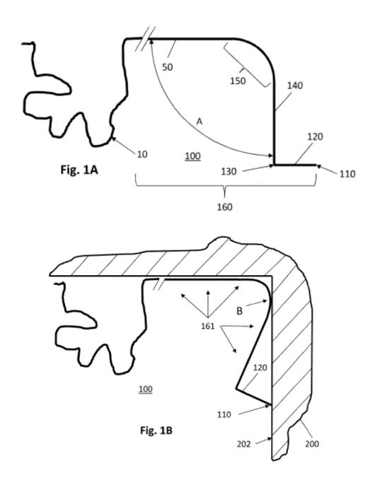
Figure 1A shows a sectional view of thermoplastic article 100 inserted within interior of upper body 200, shown in Figure 1B, prior to bending an unwanted sharp edge away from the periphery of the article. *Id.* at 6:14–34. Thermoplastic article 100 has "deflectable flange 160 formed at an edge thereof." *Id.* at 6:19–21. Deflectable flange 160 includes extension 50, bend
