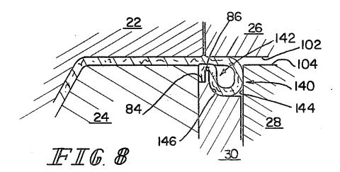
In Figure 8, an apparatus with elements including vertically upper die member 22, vertically lower die member 24, vertically upper draw pad 26, vertically lower draw pad 28, and ring 30 work in conjunction to form a blank of flexible material into a desired configuration. *Id.* at 2:59–3:2, 3:57–
