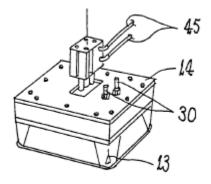
The excerpted figure above shows clackerbox 14, including clamping feet 13, water cooling pipes 30, and compressed air conduits 45 for moving feet 13 of clackerbox 14 in and out from under rim 10 of tray being formed.
