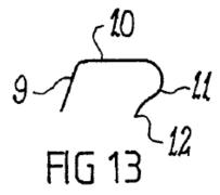
Figure 13 shows a finished tray edge with sloping sidewall 9, that has "a more rounded peripheral edge region" than that of other trays. *Id.* at 8:19–9:3, 14:15–17. The profile edge of the tray has rim 10 connected to peripheral edge region 11, which is connected to terminal edge 12. *Id.* at 14:10–13. Portelli discloses that the trays can have a rounded rectangular shape with a concave compartment formed therein. *See* Figs. 14–16.
