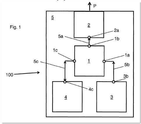
The "apparatus 100 comprises the processor 1, projector 2, [and] movement sensor 3." *Id.* at 4:34-35. The processor 1 includes an "input 1a" and an "output 1b."
