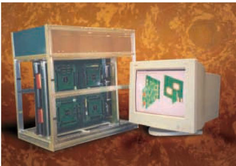
Figure 1 - Co-verification solution: Italtel FlexBench hardware with Temento Diaflex software
