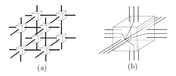
Figure 1: (a) 3D FPGA, and (b) 3D switch block.
