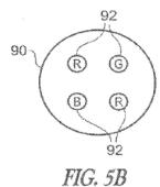
Figure 5A (upper) shows handheld lighting controller 85, and Figure 5B (lower) shows color light fitting 90 controllable by the lighting controller. *Id.* at 9:37–39. Light fitting 90 incorporates red, green, and blue lightemitting devices ("LEDs") 92. *Id.* at 9:39–40. "In the illustrated unit, there are two red LEDs, one green and one blue to provide equal maximum brightness of each color." *Id.* at 9:40–42. Lighting controller 85 has a
