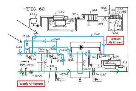
The blue exhaust air in Meckler is broken or bifurcated at least twice such that only Portion 4 loops back to the dehumidification wheel 1252, where it is heated to an elevated temperature and passed through the wheel. However, the heated exhaust air from the dehumidification wheel is vented to the atmosphere without passing through the TER device 1251. Moreover, the exhaust air in Meckler does not flow serially from the dehumidification wheel and then through the TER device.
