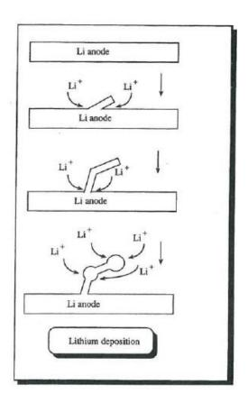
13. A large number of other research works prior to the invention of the '586 patent, as well as my own understanding of dendrite growth based on years of industry experience studying dendrite formation in lithium batteries, reflect this view of dendrite growth. Just as one example, Yamaki et al. have explained that,
