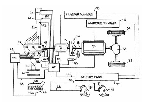
As shown, a traction motor 25 is connected to the road wheels 34 through a differential 32. A starter motor 21 is connected directly to the internal combustion engine 40. The motors 21 and 25 are functional as either motors or generators, depending on the operation of the corresponding inverter/charger units 23 and 27, which connect the motors to the battery bank 22. '347 patent, col. 26:13-27.
