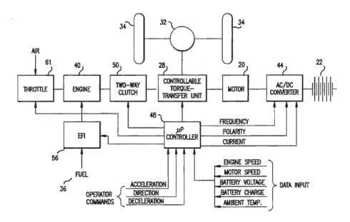
In the preferred embodiment shown in Figure 3, an internal combustion engine 40 and an alternating current (AC) motor 20 are connected to the drive wheels of the vehicle through a controllable torque transfer unit 28. The torque transfer unit receives torque from the engine 40 or motor 20 and transmits this torque to drive wheels 34. A battery 22 provides direct current
